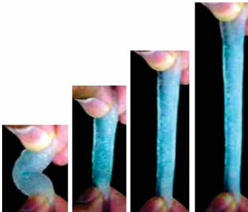
Figure 5. A third-generation superporous hydrogel hybrid with elastic property in its swollen state.
