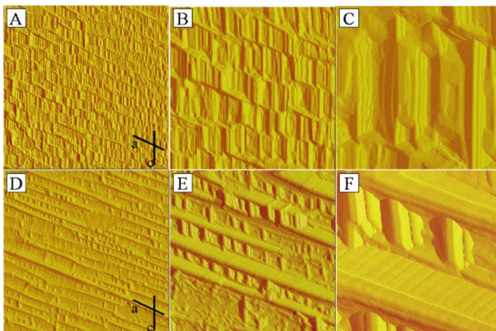
**Figure 3.** Atomic force microscopy (AFM) images of the acetaminophen (010) face etched by water. The scan sizes were  $60 \times 60 \mu\text{m}^2$  for (A) and (D),  $20 \times 20 \mu\text{m}^2$  for (B) and (E) and  $5 \times 5 \mu\text{m}^2$  for (C) and (F). (B) and (C) were zoom-in scanning of image (A) site, and (E) and (F) were zoom-in scanning of image (D) site.  $a$ - and  $c$ -axes were marked on images (A) and (D).
