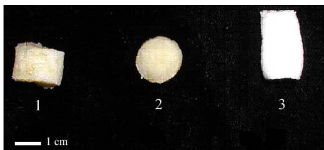
Figure 2. Photographs of PAN SPIHs synthesized using different amounts of initiators, APS and PMBS. (1) 2 mol%; (2) 1 mol%; and (3) 0.5 mol%.
