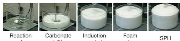
Figure 4 Steps in producing a superporous hydrogel foam.
