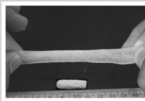
The elastic nature of the prepared, water-swollen, acrylamide-alginate hybrid hydrogel.
