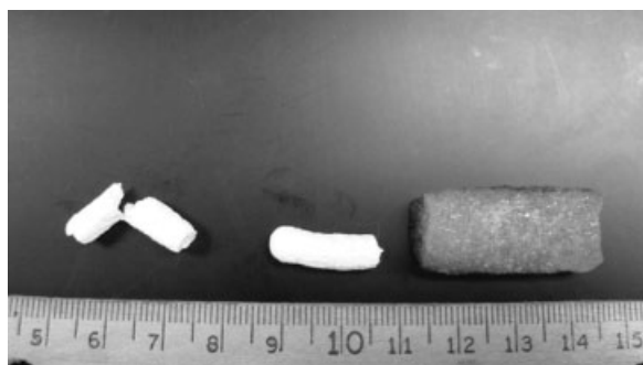
Figure 1. The final, dried hydrogel hybrid of acrylamide and alginate is rigid and brittle (left); it swells to about 10 to 15 times of its own volume in water (right).
