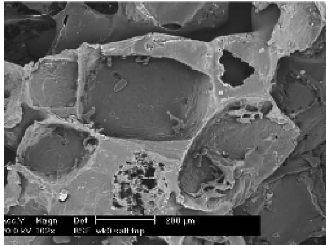
FIGURE 9.8 SEM micrograph of a foam scaffold fabricated by solvent casting/particulate leaching. PLGA disks were prepared using NaCl as a porogen. Pore shape is determined by the rectangular shape of salt particles. Scale bar = 200 \mu\text{m} . (From Reference 48 with kind permission from Elsevier.)
