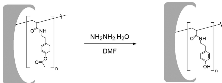
SCHEME 11.30 Deprotection of acetoxyphenol groups on a poly( N -(2-(4-acetoxyphenyl)ethyl)acrylamide)-coated polyHIPE.
