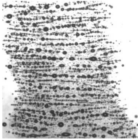
FIGURE 15.15 Chain formation in a stagnant liquid. Square wave voltage, 3.5 kV/cm horizontal electric field.
