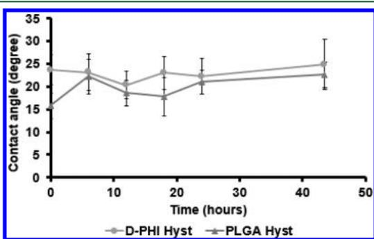
**Figure 8.** Contact angle hysteresis calculated from the advancing and receding contact angles. Data represented as mean  $\pm$  SE, with  $n = 24$  using four distinct samples and six measurements taken in different locations on each of the polymer films. PLGA hysteresis at 0 h is significantly ( $p < 0.05$ ) different from 12+ h. D-PHI hysteresis at 0 h is not significantly ( $p > 0.05$ ) different from any other time point.
