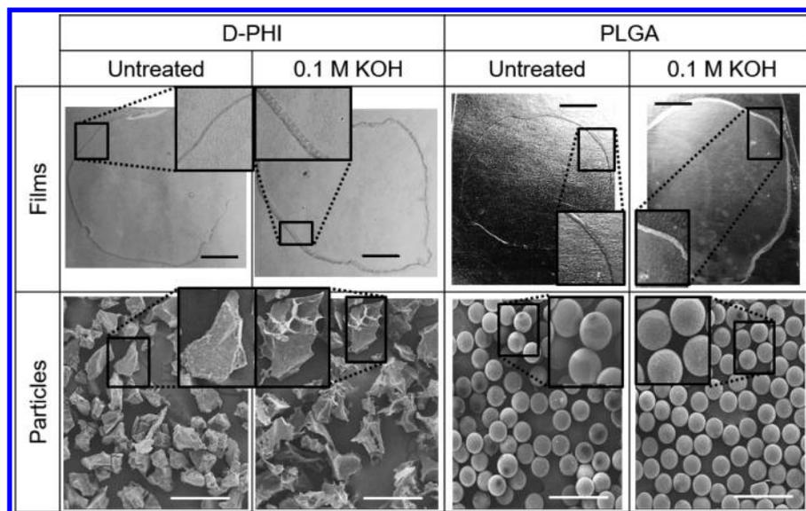
**Figure 1.** Images of films and particles of D-PHI and PLGA as native materials and after degradation with 0.1 M KOH for 18 h for D-PHI and for 6 h for PLGA. Black scale bars = 1 cm; white scale bars = 200  $\mu\text{m}$ . Zoomed-in ( $2\text{--}2.5\times$ ) images show changes over degradation that depict etching for D-PHI (more apparent for films than particles), increased cloudiness and peeling of the edges for PLGA films, but little visible differences for PLGA particles.
