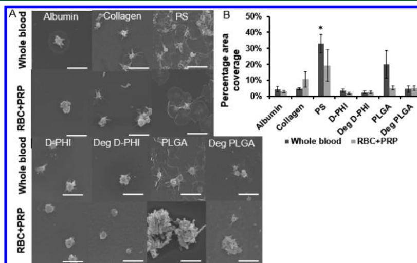
**Figure 4.** (A) Representative SEM images of platelets on film surfaces and (B) a graph showing the percentage of surface area covered by cells for each film. Data represented as mean  $\pm$  SE with  $n = 5$  experiments, each using a different blood donor (one sample per experiment, average of 10 images taken from different areas per sample). Scale bar represents  $6 \mu\text{m}$ .  $* p < 0.05$  different from all samples except PLGA.
