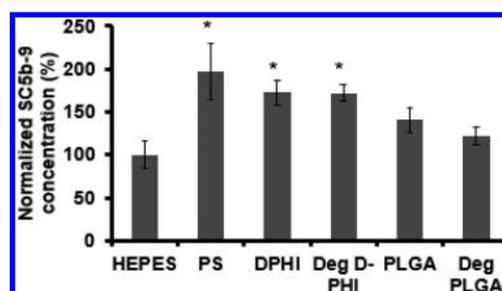
**Figure 7.** Complement activation assessed by normalized SC5b-9 concentration in serum after exposure to particles of biomaterials. HEPES acts as a normal control and heat-aggregated IgG as a positive control (not shown,  $544 \pm 121\%$ ). Data expressed as mean  $\pm$  SE,  $n = 9$ , with three different blood donors and three distinct samples for each donor. \*  $p < 0.05$  different from normal control (HEPES).
