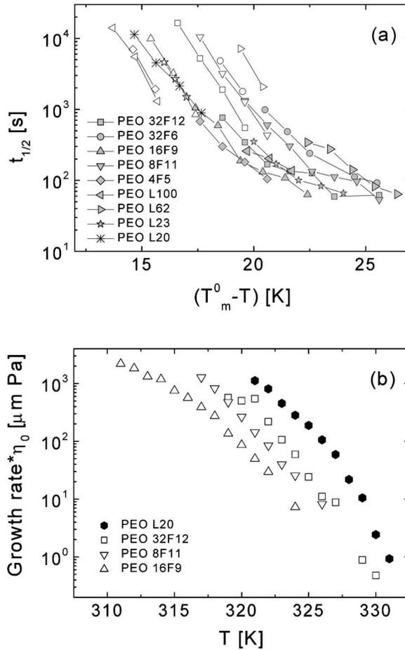
**FIG. 7.** (a) Half crystallization times for linear and star PEO samples. Empty symbols: DSC. Filled symbols: Rheology (the latter data are results of the parallel model). (b) Linear growth rates times zero-shear viscosities as functions of temperature (growth rates obtained from POM).
