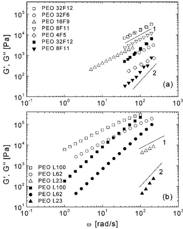
**FIG. 2.** Dynamic frequency sweeps of star PEO (a) and linear PEO (b) samples at 333 K. Filled symbols: storage modulus,  $G'$ . Empty symbols: loss modulus,  $G''$ . Lines with slopes 1 and 2 indicate the terminal scaling for  $G''$  and  $G'$ , respectively.
