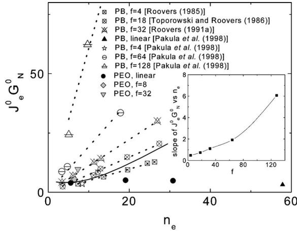
**FIG. 4.** Normalized recoverable compliance (with the plateau modulus) for linear and star PEOs as function of the number of entanglements per arm (a linear polymer is considered as having two arms). For comparison, data on PBd stars [Roovers (1985, 1991a); Toporowski and Roovers (1986); Pakula *et al.* (1998)] are also presented. The solid line is the MM theory. The dotted lines are drawn to guide the eye. Inset: The extracted slope of  $J_e^0 G_N^0$  plotted against the star functionality.
