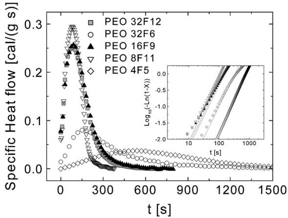
**FIG. 6.** Isothermal DSC curves of star PEO samples at 321 K (symbols in the figure). Inset: Avrami plot: Respective evolution of the relative degree of crystallinity (same symbols as in main figure). Solid lines are the fits to the data.
