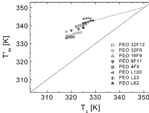
**FIG. 5.** Hoffman–Weeks plot for linear and star PEOs from isothermal DSC experiments. The solid line has a slope of 1; the dashed line shows the approximate  $T_m^0$  for sample 32F12.
