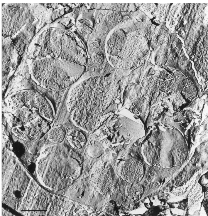
Fig. 2. Freeze fracture electron microscopy of one microsphere. Many cavities, a few of which are smooth but most of which exhibit particles, are separated by the polymer core (arrow). Bar = 2 \mu\text{m} . From [21].
