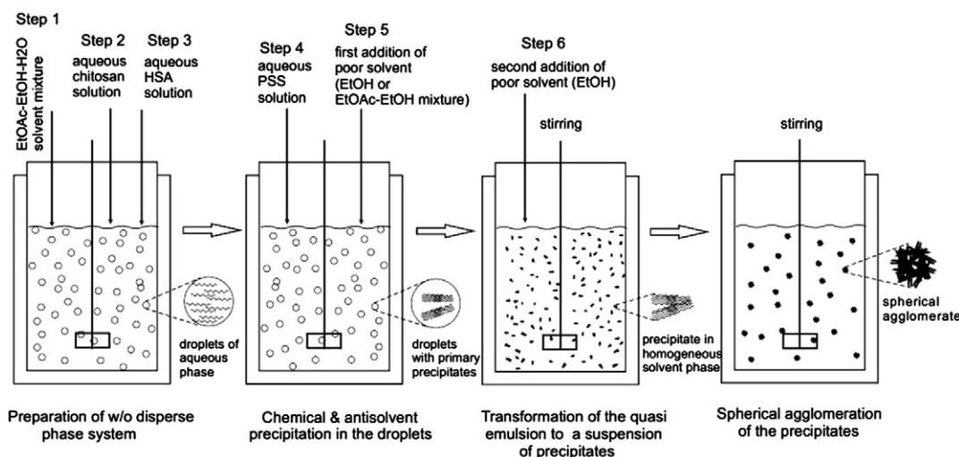
Fig. 1. Schematic diagram of the studied spherical agglomeration process.
