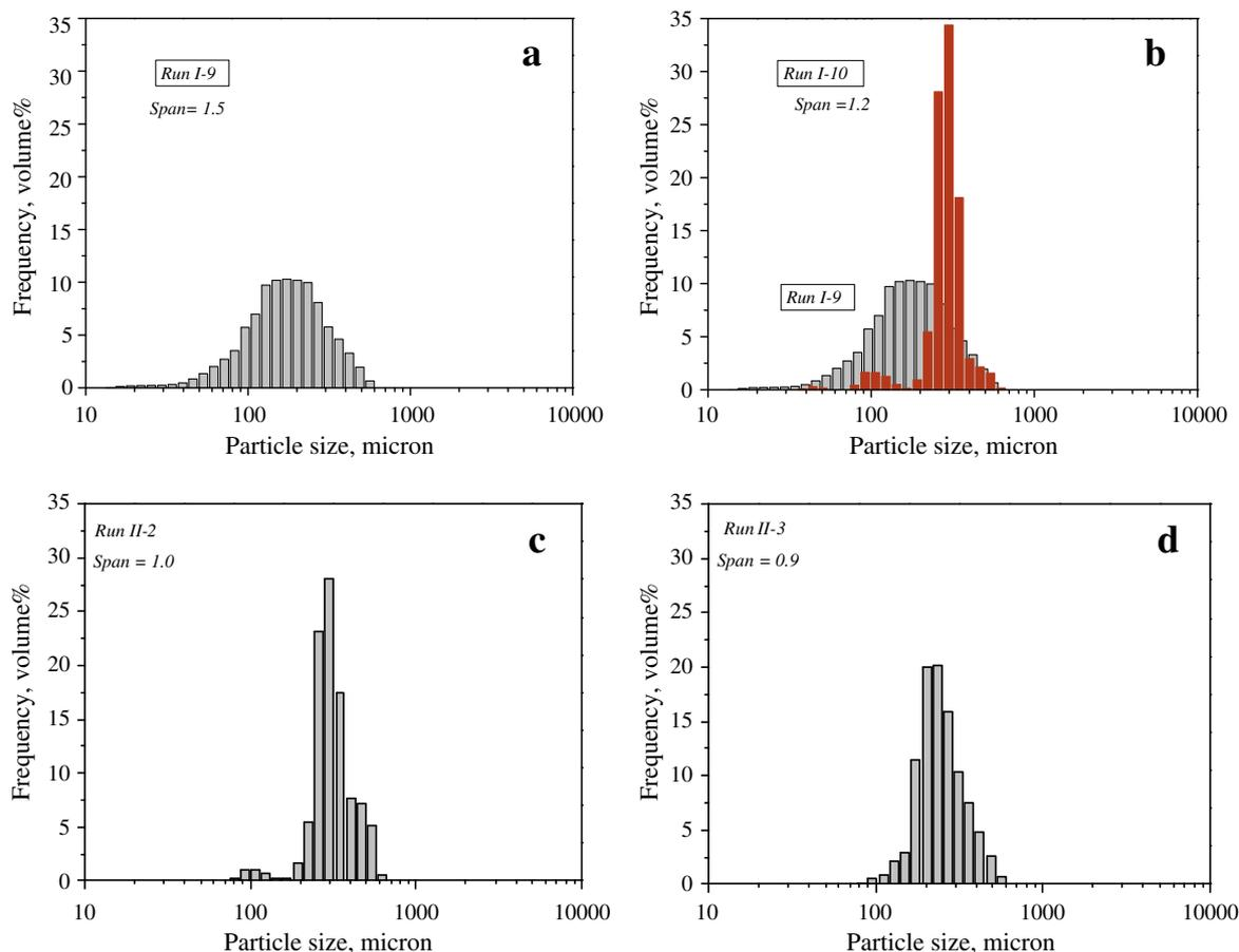
Fig. 4. Typical frequency distribution of the formed spherical agglomerates, a – run I-9, b – runs I-9 and I-10, c – run II-2, d – run II-3.
