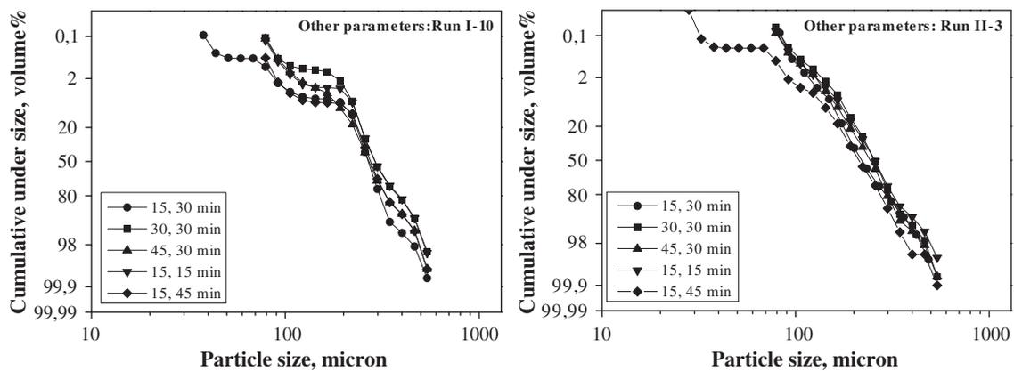
Fig. 6. Effect of stirring times applied in Steps 5 and 6 on the size distribution of the final product. The figures separated by comma in the legends denote the stirring times in minute in Steps 5 and 6, respectively.
