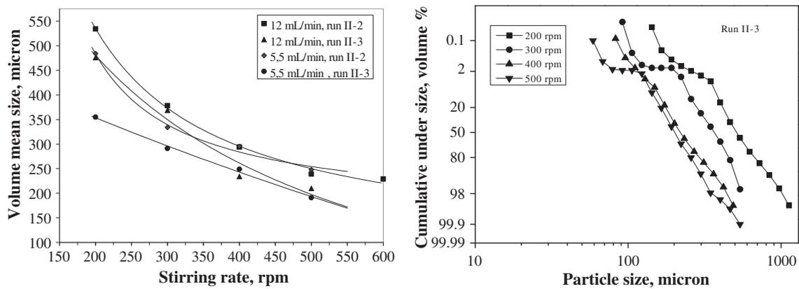
Fig. 5. Effect of stirring rate: a – volume mean size as a function of stirring intensity and the rate of poor solvent addition, b – size distributions obtained by different stirring rates of 12 mL/min. Other parameters: like Runs II-2 and II-3.
