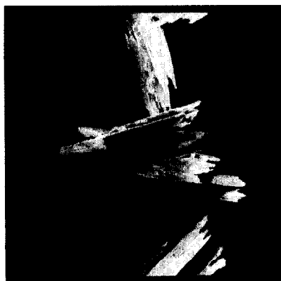
Fig. 10. C-form of stearic acid grown from acetone in quiescent system at 0.03^{\circ}\text{C min}^{-1} cooling rate in presence of 1% SPAN 60 emulsifier. Magn. \times 80 .
