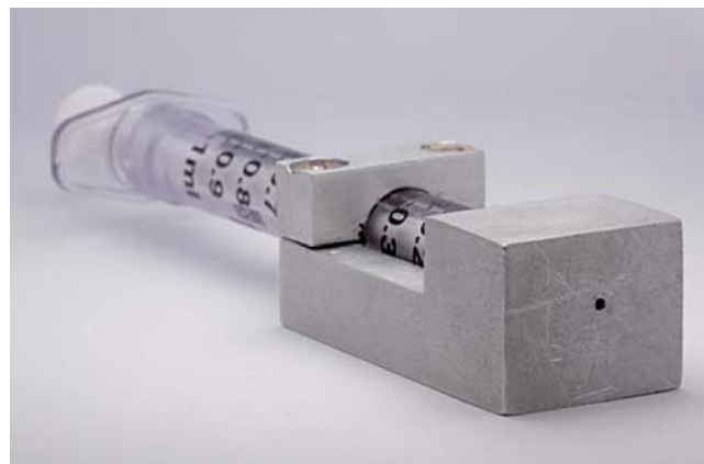
Fig. 1. Syringe-die assembly used for S-HME.
