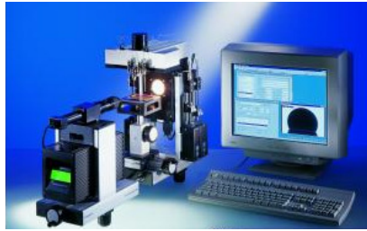
Fig. 2.2.8 Optical contact angle measuring equipment (courtesy: M/S DataPhysics Instruments GmbH).
