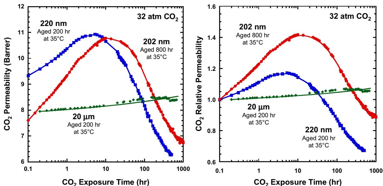
Fig. 8. Effect of aging time and thickness on long-time CO<sub>2</sub> exposure behavior.
