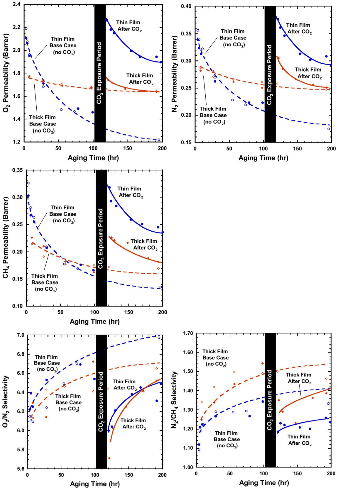
Fig. 6. CO<sub>2</sub> conditioning effects. (◇) Thin film base case, (◆) thin film with CO<sub>2</sub> exposure, (○) thick film base case, (●) thick film with CO<sub>2</sub> exposure. The CO<sub>2</sub> exposure period followed the procedure outlined in Section 3.2.
