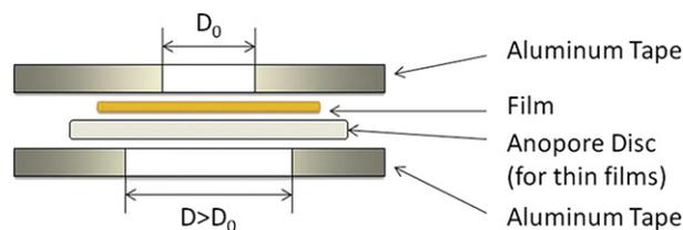
Fig. 1. Film masking schematic.
