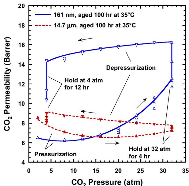
**Fig. 3.** CO<sub>2</sub> permeability hysteresis for thin and thick films with identical prior thermal history. Each film proceeds through four steps: 1. Pressurization from 2 atm to 32 atm, spending 10 min at each intermediate pressure; 2. Hold at 32 atm for 4 h; 3. Depressurization from 32 atm to 4 atm, spending 10 min at each intermediate pressure; 4. Hold at 4 atm for 12 h.
