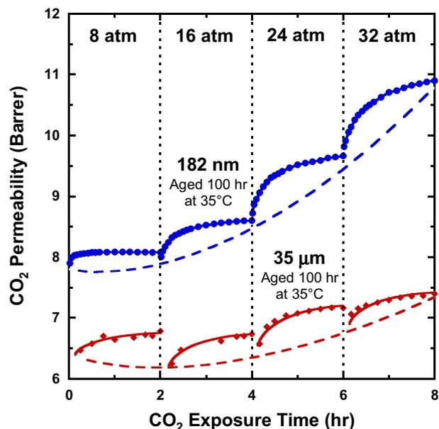
**Fig. 4.** Short time experiments for thin and thick films with identical prior thermal history.
