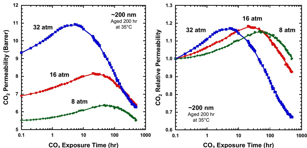
Fig. 7. Effect of long-time CO<sub>2</sub> exposure at constant pressure for thin films with identical thickness and prior thermal history.
