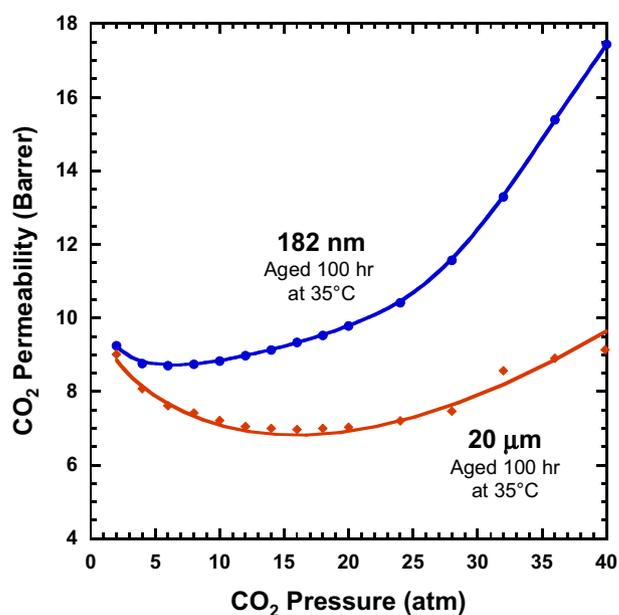
Fig. 2. CO<sub>2</sub> plasticization pressure curves for thin and thick films with identical prior thermal history. The thin and thick films spent 3 and 10 min, respectively, at each intermediate pressure.
