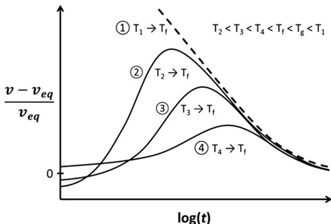
Fig. 9. Generalization of the Kovacs temperature jump experiment for glassy polymers. The response shows the deviation of sample volume ( $v$ ) from its equilibrium volume ( $v_{eq}$ ) at temperature  $T_f$  versus the time the sample has been at  $T_f$  following the various thermal histories explained in the text.
