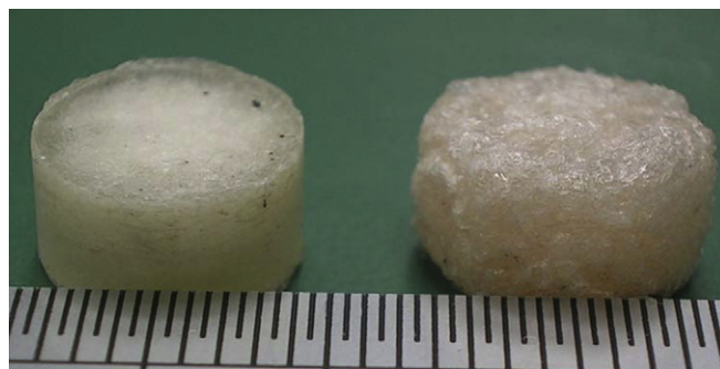
Fig. 5. Photograph of antibiotic composites after \gamma irradiation (left) and ethylene oxide treatment (right).
