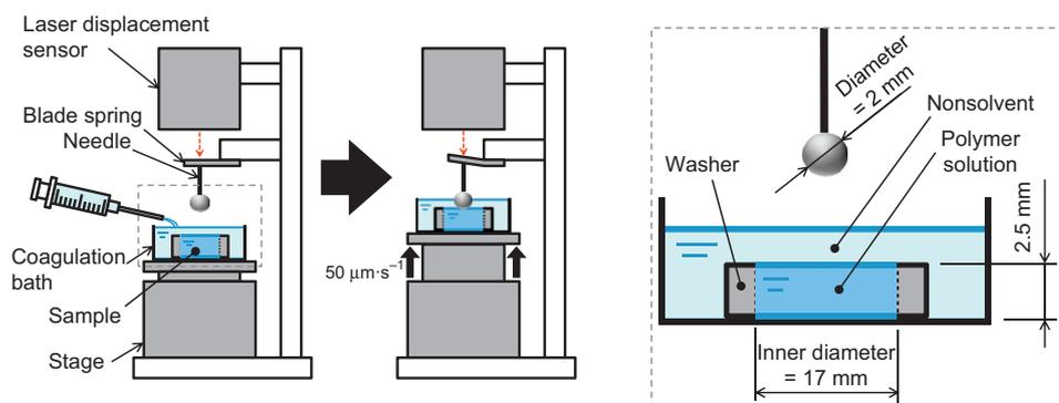
Fig. 1. Diagram of stiffness measurement apparatus.
