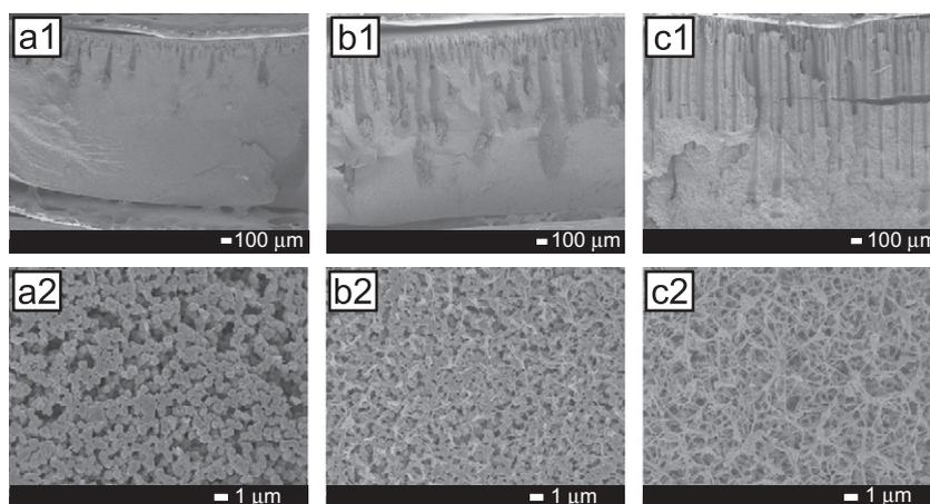
Fig. 9. SEM images of membranes with a, no additives; b, PEG; c, PVP. 1, cross-section; 2, outer surface.
