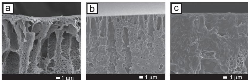
**Fig. 7.** Cross-sectional SEM images near the outer surfaces with different PVDF molecular weights. (a)  $M_w=136,000$ ; (b)  $M_w=176,000$ ; and (c)  $M_w=271,000$ .
