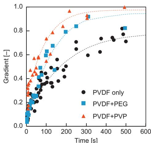
**Fig. 8.** Time variations in gradient without and with addition of PEG and PVP to polymer solution.
