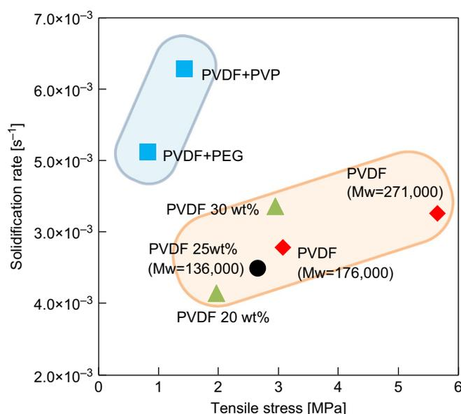
Fig. 10. Relationship between the solidification rate of the polymer solutions and ultimate tensile stress and comparison of factors that influenced the solidification rate. Black circle, raw PVDF only (control); green triangles, effect of polymer concentration; red diamonds, effect of molecular weight; blue squares, effect of additive. (For interpretation of the references to color in this figure caption, the reader is referred to the web version of this article.)
