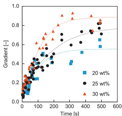
**Fig. 4.** Time variations in gradient with different polymer concentrations. Dot lines show the experimental tendencies.
