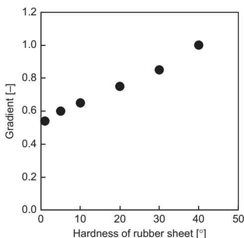
**Fig. 3.** Comparison of gradients for various rubber sheet hardnesses.
