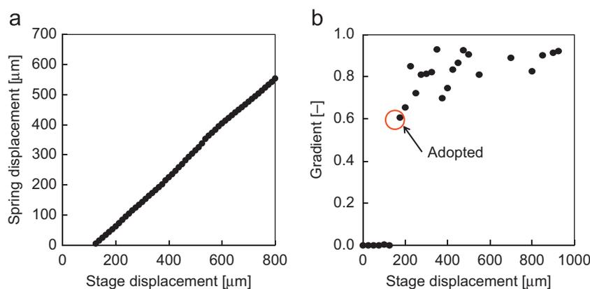
**Fig. 2.** Relationship between (a) spring displacement and stage displacement; and (b) gradient of spring displacement and stage displacement in the case of a rubber sheet hardness of  $10^\circ$ .
