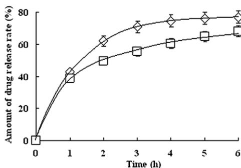
Fig. 4. Plot of the release rate of RFP from RFP/PLGA microspheres produced by using the DCM and CR by using the membrane emulsification technique.  $\diamond$ , DCM;  $\square$ , CR.
