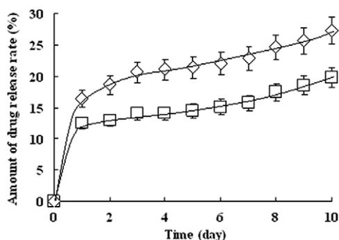
Fig. 6. Plot of the release rate of BLD from the BLD/PLGA microspheres prepared by using the membrane emulsification technique.  $\diamond$ , DCM;  $\square$ , CR.
