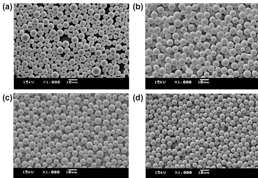
**Fig. 2.** SEM images of the RFP/PLGA microspheres prepared by using the membrane emulsification technique. (a) Sample 12, (b) sample 15, (c) sample 17, (d) sample 18.
