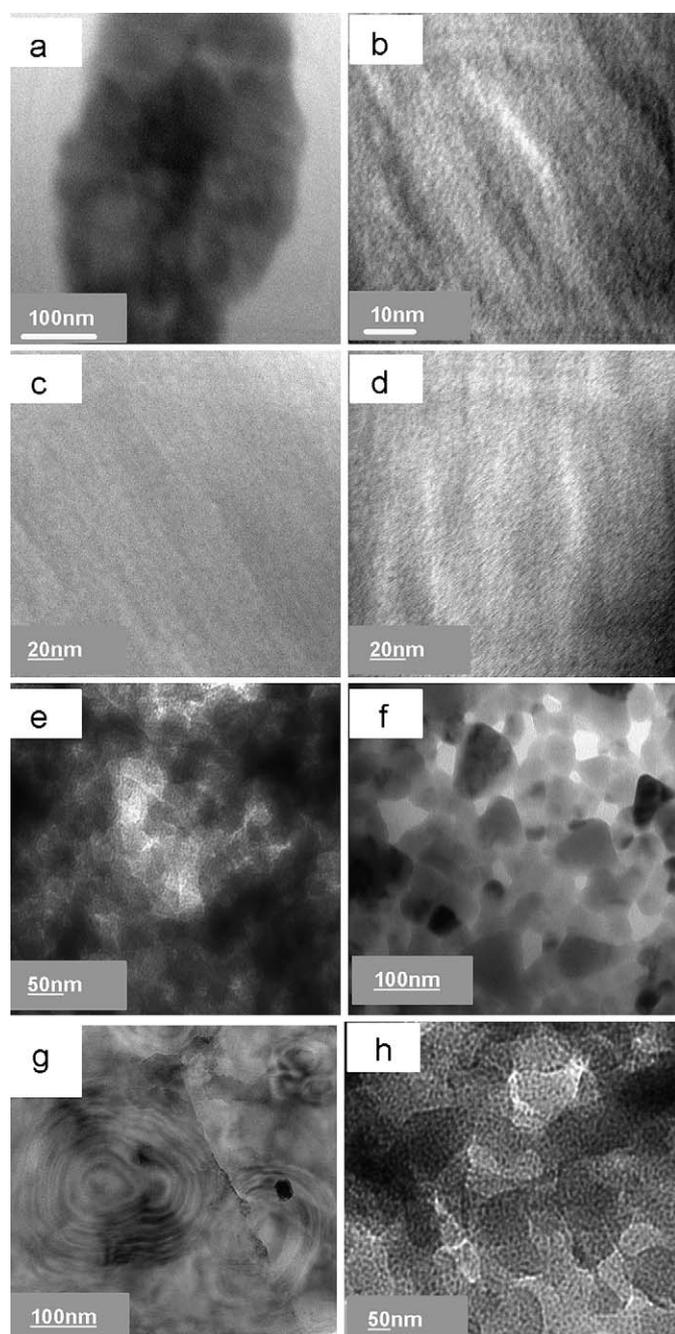
**Fig. 5.** HRTEM of SMA powder irradiated at (a) 8.25 Gy/min shows clustering (b) 17.29 Gy/min with much reduced clustering (c) 20.01 Gy/min showing optimum characteristics. (d) 25.00 Gy/min is near to desired morphology. RISUG<sup>®</sup> precipitates (e) 8.25 Gy/min with coagulated appearance (f) 17.29 Gy/min show less coagulation. (g) 20.01 Gy/min illustrates ideal plaque like structure. (h) 25.00 Gy/min may also be accepted.
