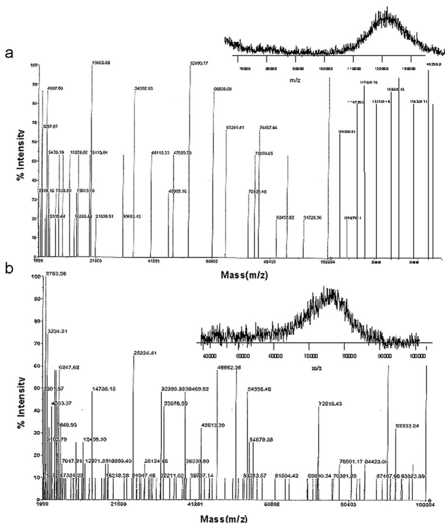
**Fig. 2.** MALDI-TOF based molecular weight analysis of SMA. (a) Molecular weight ( $M_n$ ) of  $M_3$  sample irradiated at dose rate 8.25 Gy/min with total dose 2.2 kGy is 119 kDa and distribution pattern ranges from 70 to 130 kDa. (b) Molecular weight ( $M_n$ ) of  $M_{11}$  sample irradiated at dose rate 20.01 Gy/min with total dose 2.2 kGy is 72 kDa and distribution pattern ranges from 40 to 100 kDa.
