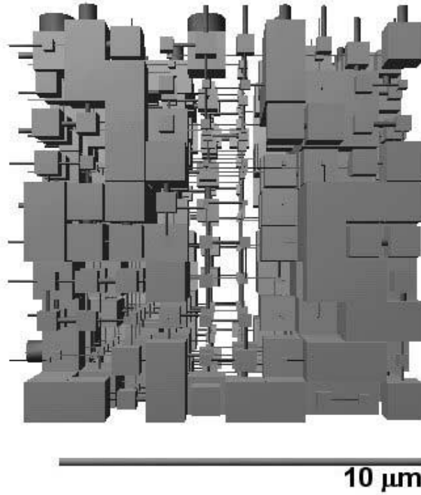
Figure 16 - Modelled structure of a high T_g latex-based coating applied with rod 2 - here the picture is different with large pores retained in the coating illustrating the resistance to shrinkage.
