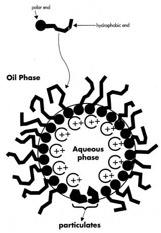
**Fig. 2** Water-in-oil emulsions. Water droplet in oil showing stabilization by surfactants and particulates. Modified from Christopher (1993).
