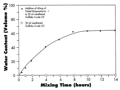
**Fig. 10** Effect of nickel porphyrin to weathered Gullfaks crude oil. Seawater (300 ml) was mixed with 30 ml of weathered Gullfaks crude oil (non-emulsion forming oil) and 40 mg of nickel porphyrin. No emulsion was formed when nickel porphyrin was added to non-weathered oil. Oil was weathered by setting it outside in a beaker for 3 days before use.
