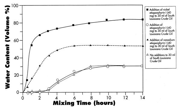
**Fig. 9** Effect of porphyrin additions on the formation of oil-in-water emulsions. Seawater (300 ml) was mixed with 30 ml of South Louisiana crude oil (non-emulsion forming oil) and 40 mg of one of the porphyrins. The mixture was placed on a rotating apparatus and the water content of the emulsion formed was noted at the different times.
