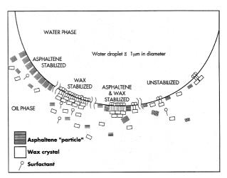
Fig. 3 Schematic diagram showing a water emulsion droplet in oil which is stabilized by asphaltenes, surfactants and waxes. An unstabilized region is shown where there is formation of an incomplete barrier. Modified from MacKay (1987).
