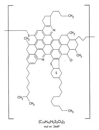
Fig. 5 Hypothetical structure of a petroleum asphaltene. Modified from Speight and Moschopedis (1981).
