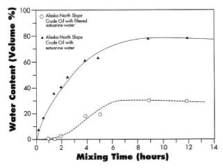
Fig. 4 Effect of seawater particulates on formation of water-in-oil emulsion by Alaska North Slope crude oil. Seawater (300 ml) either filtered (0.45 µm filter) or unfiltered was mixed with 30 ml of oil on a rotating apparatus and the water content of the emulsion formed was noted at the different times.
