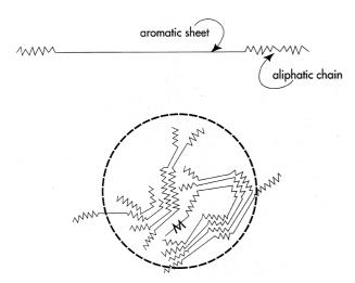
Fig. 6 Asphaltene micelle. Metal porphyrin (M) is a coordination center for several clusters. Modified from Yen (1981) and Speight and Moschopedis (1981).
