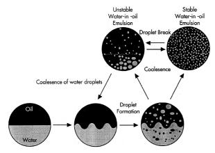
Fig. 1 Formation of water-in-oil emulsions. Modified from Lewis and Walker (1993).
