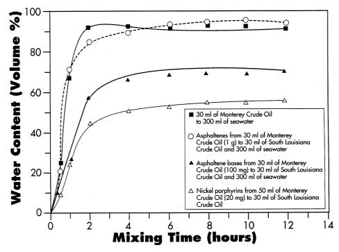
Fig. 8 Emulsion formation by monterey crude oil and by addition of various fractions of monterey crude oil to south Louisiana crude oil (non-emulsion forming oil). Sea water (300 ml) was mixed with oil, oil fraction and/or porphyrins on a rotating apparatus and the water content of the emulsion formed was noted at the different times.
