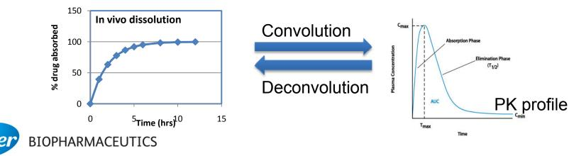
Deconvolution is the reverse process of convolution
