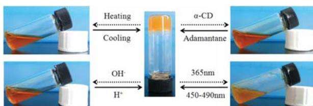
**Figure 1.** Photographs of the reversible gel–sol transition of LPF2-PPI hydrogel triggered by multiple stimuli (temperature, pH, host–guest interaction, and photoirradiation, respectively).
