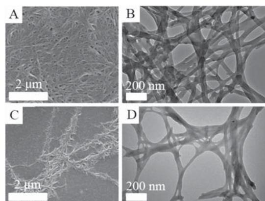
**Figure 2.** SEM images of LPF2-PPI gel before (A) and after (C) UV irradiation (365 nm) for 30 min. TEM images of LPF2-PPI gel before (B) and after (D) UV exposure for 30 min.
