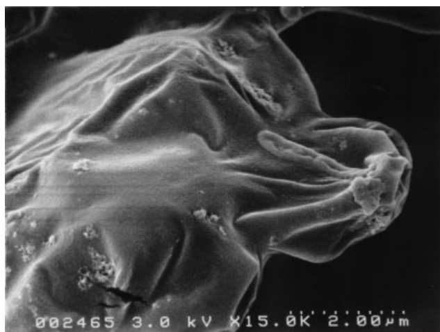
Figure 6. SEM photo of the cell/polymer constructs showing the attachment of the cells on the surfaces of the biodegradable scaffolds ( \times 30 ).
