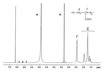
Figure 4.  $^{1}$ H-NMR spectra of pure PAA(CD<sub>3</sub>OD as solvent). \*Attributed to CH<sub>3</sub>OH and H<sub>2</sub>O in CD<sub>3</sub>OD.
