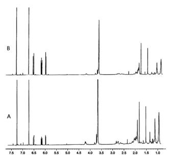
**Figure 6.** <sup>1</sup>H NMR spectra of heteroarm star-shaped polymers obtained at different monomer conversions in CDCl<sub>3</sub>. (A) 26.45% AA conversion; (B) 56.62% AA conversion.
