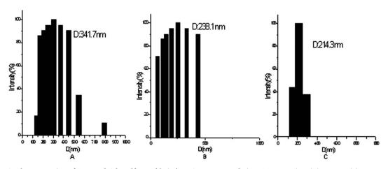
Figure 9. DLS columnar section of A, B, and C by self-assembly in l% KOH aqueous solution. AA conversion: (A) 26.45%, (B) 56.62%, (C) 96.0%.
