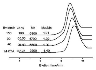
**Figure 3.** GPC curves of products obtained at different monomer conventions in THF at  $60^{\circ}$ C. Reaction conditions: [AA] = 2.4 mol/L; m(S-PMMA) = 0.66 g (0.2 mmol), m(AA) = 4 g m(AIBN) = 0.01–0.015 g.
