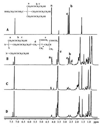
Figure 2. <sup>1</sup>H-NMR spectra of PETMP and PMMAs obtained with the ratio of MMA to PETMP to be 70/1. (A) PETMP; (B) PMMAs obtained at 37.75% conversion; (C) PMMAs obtained at 54.96% conversion; (D) PMMAs obtained at about 100% conversion.
