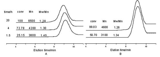
Figure 1. GPC curves of PMMAs obtained at different monomer conventions in benzene at 70°C. Reaction conditions: [MMA] = 3 mol/L; (A) [MMA]: [PETMP]: [AIBN] = 70:1:0.3; (B) [MMA]: [PETMP]: [AIBN] = 50:1:0.3.
