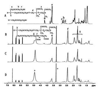
**Figure 5.** <sup>1</sup>H-NMR spectra of M-CTA and heteroarm star-shaped polymers obtained at different AA conversions in CD<sub>3</sub>OD: (A) M-CTA; (B) 29.48% AA conversion; (C) 65.56% AA conversion; (D) 96.0% AA conversion. \*Attributed to CH<sub>3</sub>OH and H<sub>2</sub>O in CD<sub>3</sub>OD.
