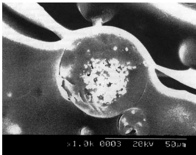
Fig. 1. Scanning electron micrograph of cross-section of multi-reservoir type microspheres (Matsumoto et al., 1997).
