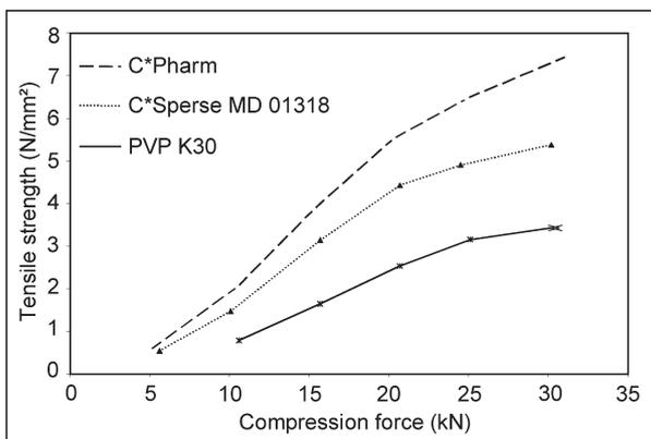
Figure 4 - Compression profile of different maltodextrin grades in comparison with PVP K30 (0.5% magnesium stearate and 0.25% SiO<sub>2</sub>)
