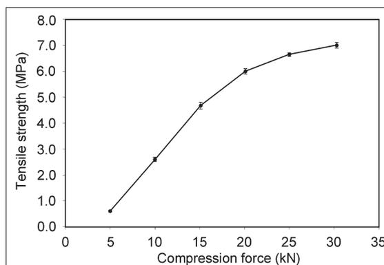
Figure 2 - Compression profile of C☆Pharm 93000. Lubricated with 0.5% magnesium stearate and with the addition of 0.25% SiO<sub>2</sub>
