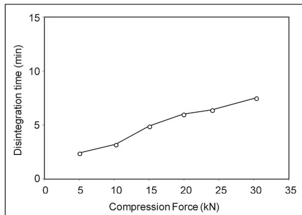
Figure 3 - Disintegration profile of C☆Pharm 93000. Lubricated with 0.5% magnesium stearate and with the addition of 0.25% SiO<sub>2</sub>
