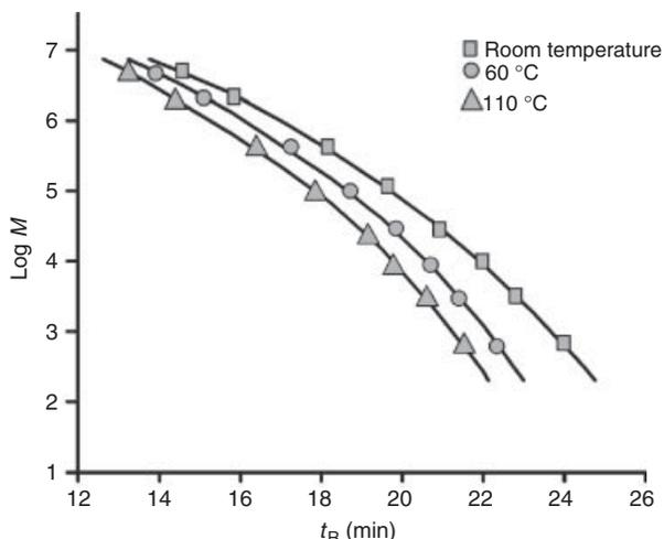
**Figure 17.5** Effect of column temperatures on calibration curves of eight PS standards. *Source:* Reprinted with permission from Cho H, Park S, Ree M, Chang T, Jung JC, Zin WC. *Macromol Res* 2006;14(3):383 [27]. Copyright 2006 The Polymer Society of Korea.
