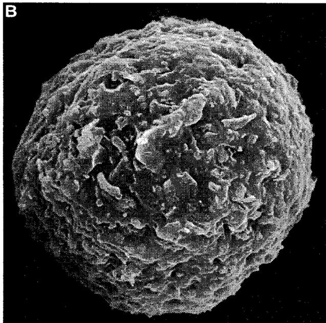
**Fig. 3.** A. Cartoon of internal structure of PLGA microsphere. The particles of rhGH:Zn complex and zinc carbonate, both of which are approximately 3 microns in diameter, are embedded into the solid PLGA matrix. The microspheres analyzed in our study were 15% w/w rhGH:Zn and between 0 and 6% w/w zinc carbonate. B. Scanning electron micrograph of a PLGA microsphere (Formulation II).
