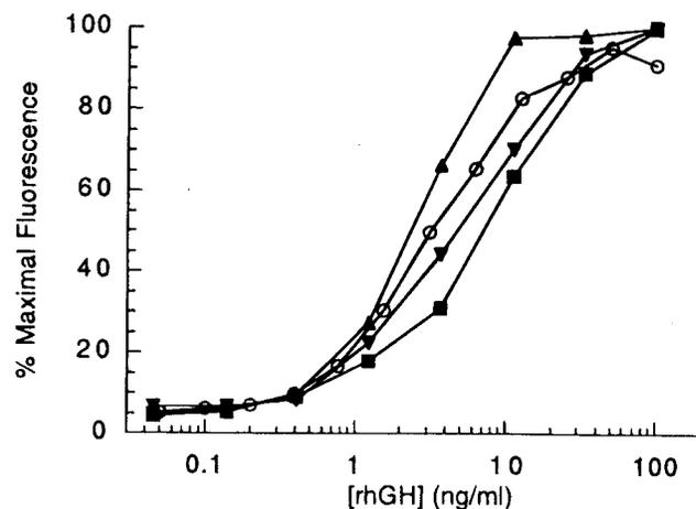
**Fig. 4.** Bioactivity of extracted rhGH measured by proliferation of a cell line expressing the hGH receptor. Microsphere Formulations I (■), II (▲) and III (▼) were incubated for 14 days in aqueous buffer and the concentration of protein released between days 10 and 14 was determined by SEC. Dilutions of these, as well as unencapsulated protein (○), were incubated with the cell line, Alamar Blue added, and fluorescence, which is an indication of cell number, was measured.
