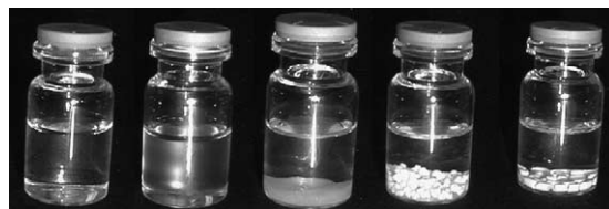
Fig. 1. States of decreasing solubility corresponding to the solubility numbers from 2 to 6 (left to right).
