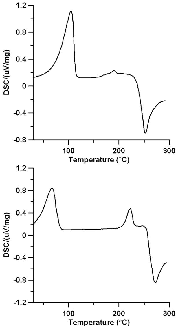
**Figure 1.** DSC trace of naloxone hydrochloride dihydrate (top) and naltrexone hydrochloride tetrahydrate (bottom) obtained with a heating rate  $5^\circ\text{C}/\text{min}$ . The sample mass was 13.2 mg for naloxone hydrochloride dihydrate and 18.2 mg for naltrexone hydrochloride tetrahydrate.
