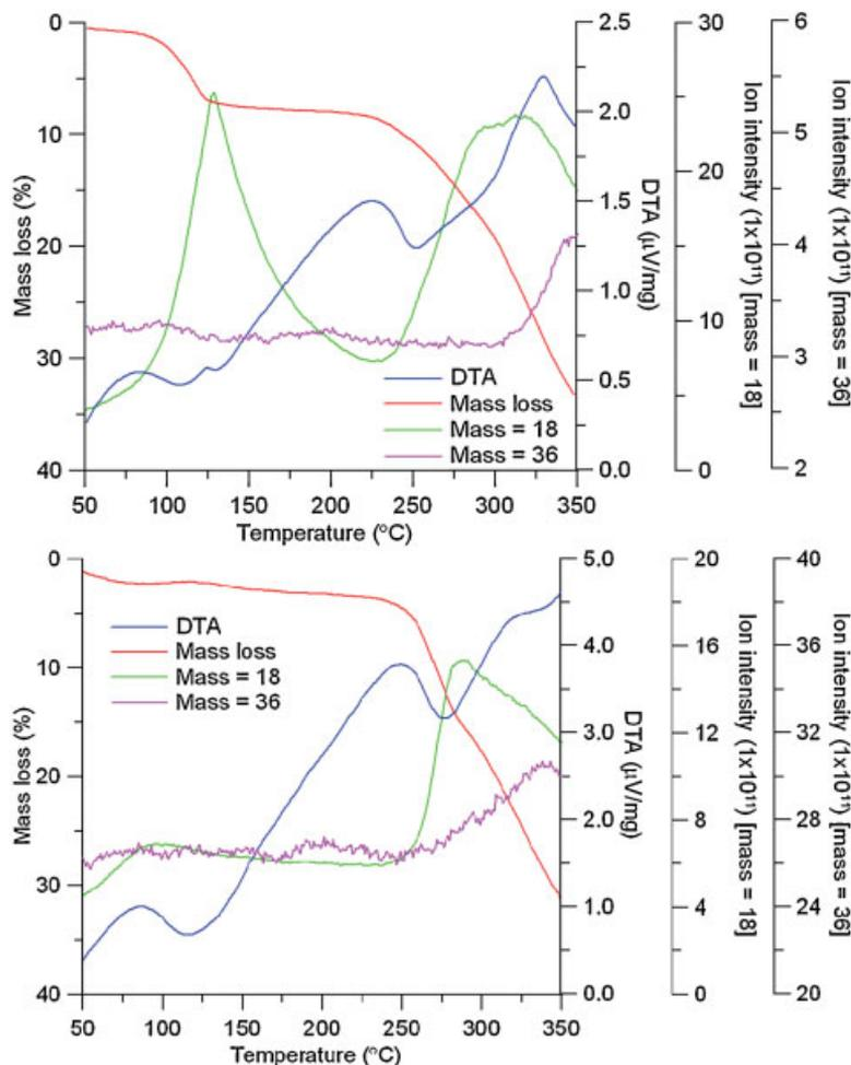
**Figure 2.** DTA trace and TG/MS profile of naloxone hydrochloride dihydrate (top) and naltrexone hydrochloride tetrahydrate (bottom) obtained with a heating rate 5°C/min. The sample mass was 13.8 mg for naloxone hydrochloride dehydrate and 6.8 mg for naltrexone hydrochloride tetrahydrate. The DTA (solid line, the mass loss (dashed line)) and the ion current for mass 18 (chain dotted line) are shown.
