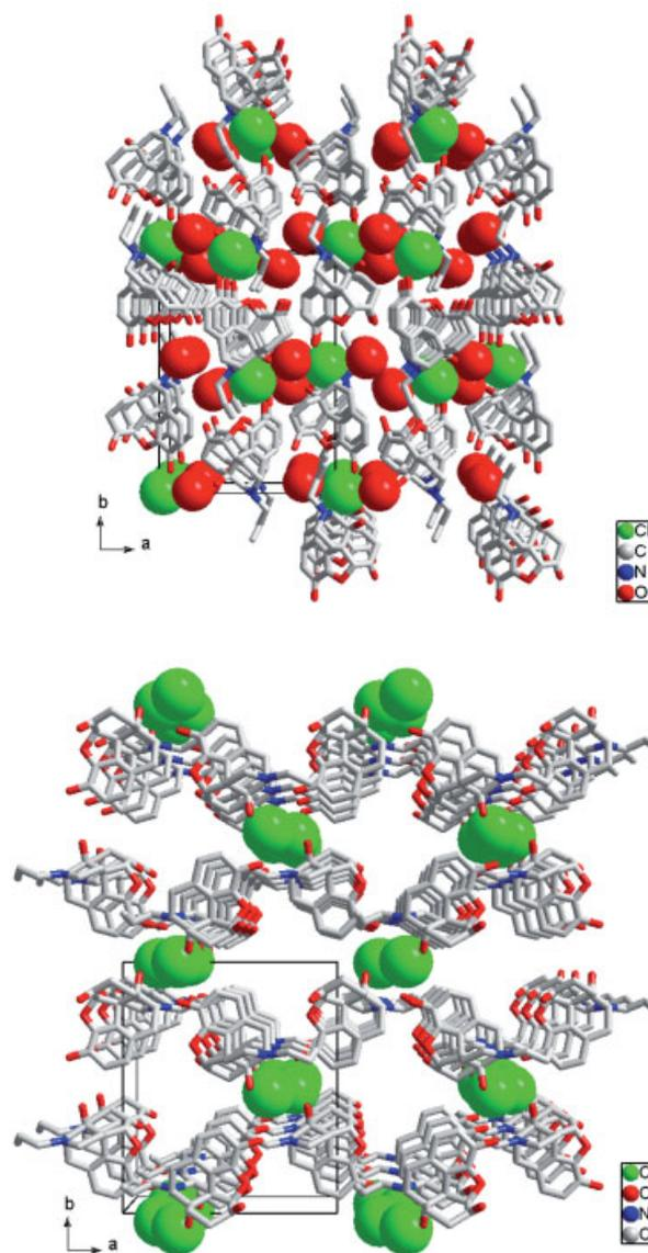
**Figure 5.** Representations of the packing of the molecules of naloxone hydrochloride dihydrate<sup>6</sup> and naloxone hydrochloride anhydrous in a projection along  $c$ -axis (blue: O atoms, green N-, or Cl-(enlarged) atoms, black: C-atoms) using the coordinates as derived from the simulated annealing procedure. Hydrogen atoms are omitted for clarity.
