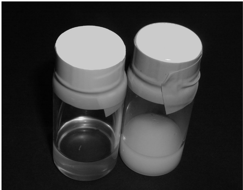
Fig. 3. The appropriate amount of additives improved the turbidity of the oil phase containing PLGA, insulin, and ZnO. Insulin was present in the oil phase containing PLGA as a dispersed suspension (right). The appropriate amount of distilled water improved the turbidity (left). The optical density of this suspension was reduced from 3.8 to 1.5 at 400 nm. The appropriate amount of ethanol and glycerin had the same effect.
