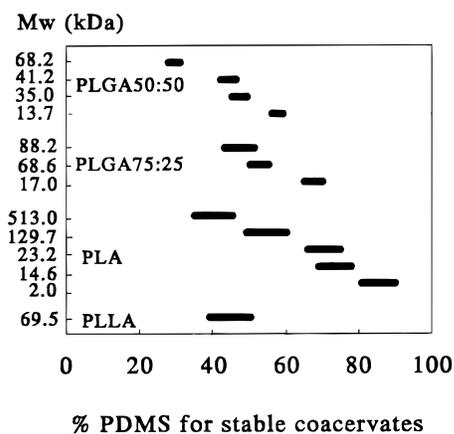
Figure 2—Amounts of PDMS (1070 mPa s) defining the area of stable coacervate droplets for different polymer types and molecular weights.
