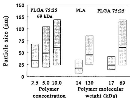
Figure 5—Effect of polymer type, molecular weight, and initial concentration in the solvent on the particle size distribution of microspheres. The 1070 mPa s PDMS was used for phase separation. The bars represent the 10–90% undersize diameters and the bold line inside the bar the average particle size.
