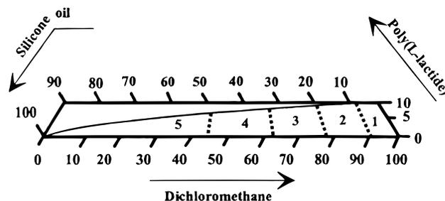
**Figure 1—Phase diagram of poly(L-lactide) characterizing the phase separation process in a DCM/PDMS mixture. The dotted lines represent the boundaries between the stages 1–5, which can be microscopically distinguished during coacervation.**
