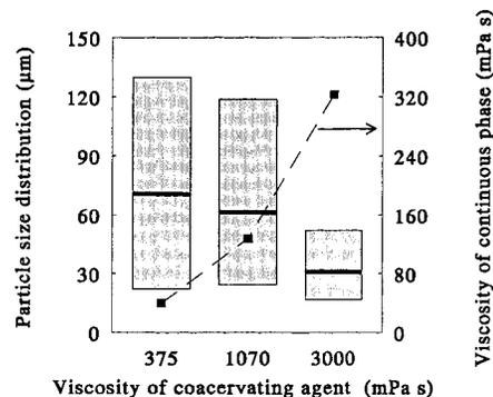
Figure 4—Effect of the coacervating agent (PDMS) viscosity on the viscosity of the continuous phase (dashed line) and the volume weighted particle size distribution of 68.6 kDa PLGA 75:25 microspheres. The bars represent the range of 10–90% undersize diameters and the bold line inside the bar the average particle size.
