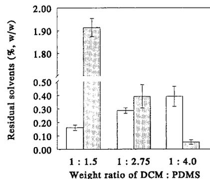
Figure 3—Residual processing liquids in 14.6 kDa D,L-PLA microspheres obtained from different coacervation compositions: polymer solvent DCM (unfilled) and hardening agent OMCTS (filled).
