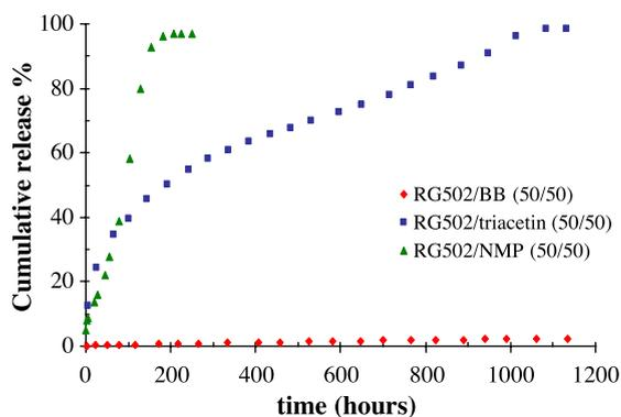
Fig. 3. The amount of solvent released into the buffer as a function of time, PLGA (RG502) solutions in vitro in pH 7.0 buffer at 37 °C: the formulation is PLGA/solvent=50/50 by weight.
