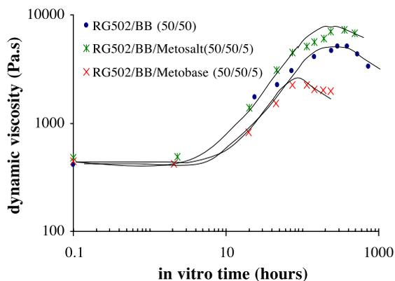
Fig. 7. The flow properties of PLGA (RG502)/benzyl benzoate solution with/without drug during in vitro: the formulation is PLGA/BB/drug=50/50/5 by weight.
