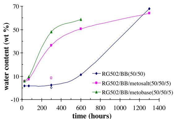
Fig. 4. Water content in RG502/BB depots with/without drugs during in vitro: filled legends represent the water content in the whole depot (including core and surface), while unfilled □ represents the water content in the core of RG502/BB/metosalt system, unfilled ◇ represents the water content in the core of RG502/BB system (only at one time point).
