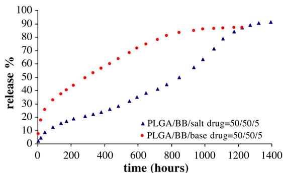
Fig. 8. Release kinetics of metoclopramide salt and base from PLGA (Resomer 502)/benzyl benzoate system: the formulation is PLGA/BB/drug=50/50/5 by weight.
