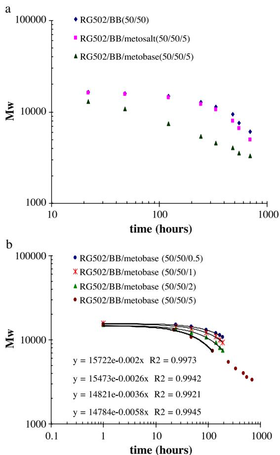
Fig. 1. (a) In vitro degradation of PLGA (RG502)/benzyl benzoate solution with/without drug, where drugs are metoclopramide salt and base, and the formulation is PLGA/BB/drug=50/50/5 by weight. (b) Effect of metoclopramide base loadings on the degradation of PLGA (RG502)/benzyl benzoate formulations: the pseudo first-order kinetics analysis is shown for different drug loadings concentration within the first 200 h.
