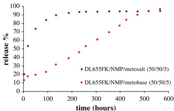
Fig. 9. Release kinetics of metoclopramide salt and base from PLGA (DL655FK)/NMP solution system: the formulation is PLGA/BB/drug=50/50/5 by weight.
