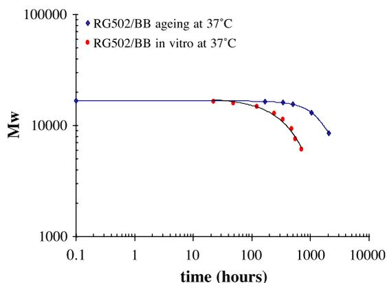
Fig. 2. The change of PLGA mass molecular weight, PLGA (RG502)/benzyl benzoate (50/50) solution aged and in vitro at 37 °C.
