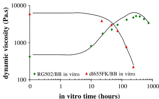
Fig. 6. Viscosity change of PLGA/benzyl benzoate (50/50) solutions during in vitro: different polymers compared.
