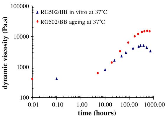
Fig. 5. The flow properties of PLGA (RG502)/benzyl benzoate solution during in vitro and upon ageing at 37 °C: the formulation is PLGA/BB=50/50 by weight.
