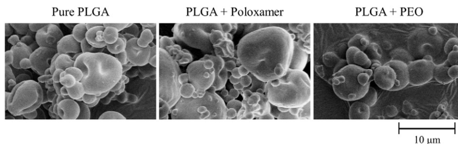
Fig. 2. SEM pictures of spray-dried prilocaine loaded microparticles before exposure to phosphate buffer pH 7.4. All formulations contained 1% drug. The (optional) Poloxamer/PEO content was 9.9%.
