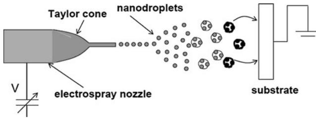
**Fig. 37.9** Electro spraying technique for producing nanoparticles by spray methods. (Reprinted from [16] with permission. Copyright 2009 Bentham Science Publishers)
