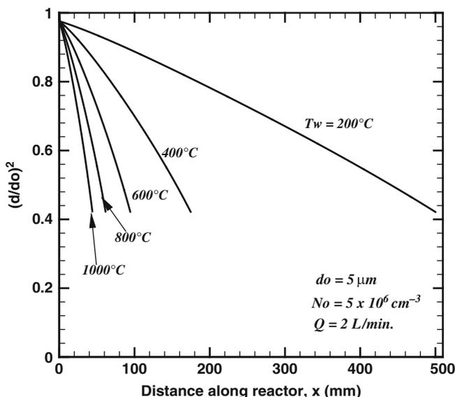
**Fig. 37.3** Non-dimensional droplet diameter variations as a function of distance from the reactor inlet for various  $T_w$ , for given  $d_0$ ,  $N_0$ ,  $Q$ ,  $RH_0$ , and  $C_0$ . Reactor inlet gas and droplet temperatures are 25°C  $RH_0 = 10\%$ , and initial solute concentration  $C_0 = 2$  M. (Reprinted from [10] with permission. Copyright 2009 of Taylor & Francis)
