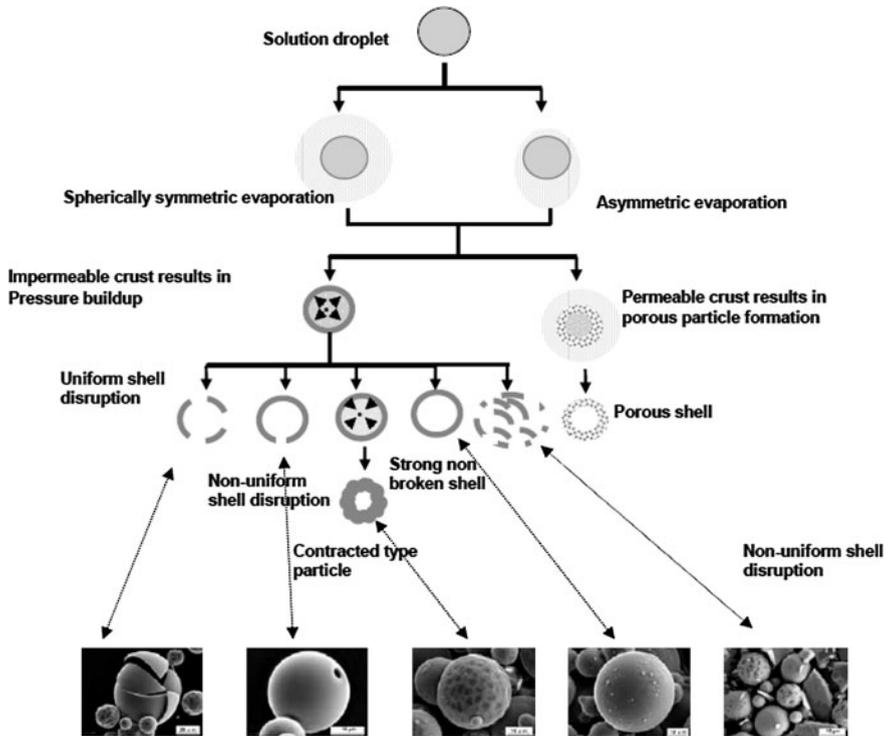
**Fig. 37.8** Different possibilities for hollow particle formation during spray drying/pyrolysis. Type (a) uniform shell disruption, type (b) non-uniform shell disruption, type (c) contracted shell particle, type (d) non-disrupted smooth surface particle, type (e) non-uniform shell disruption, and type (f) porous particle. (Reprinted from [13] with permission. Copyright 2007, American Society of Mechanical Engineers)
