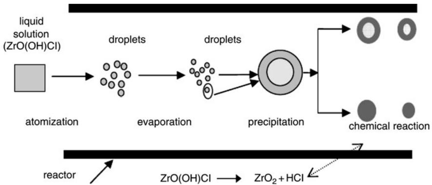
**Fig. 37.1** Basic steps of spray pyrolysis method for zirconium hydroxychloride ( $ZrO(OH)Cl$ ). Once the ( $ZrO(OH)Cl$ ) powders are relatively dried, they decompose to  $ZrO_2$  and  $HCl$  gas.  $ZrO_2$  powders remain in the collector and  $HCl$  gas goes to the carrier gas. (Reproduced from [1] with permission. Copyright 2006 Institute of Physics)
