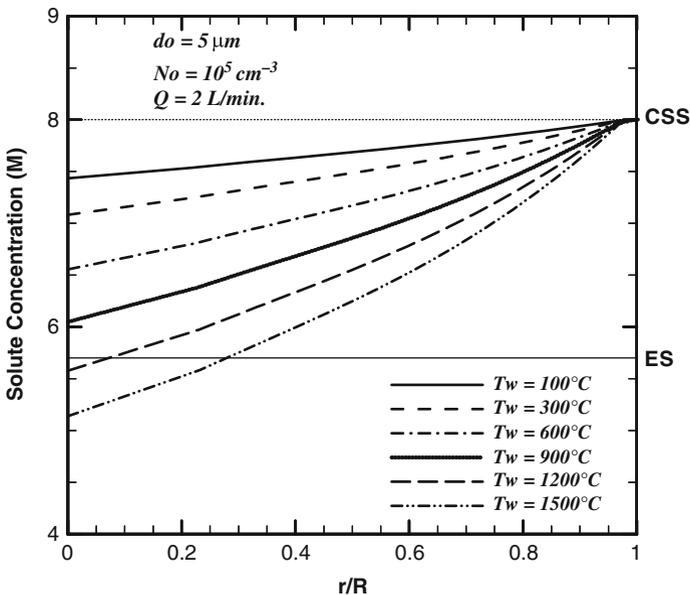
**Fig. 37.2** Solute concentration profile within the droplet for various wall temperatures for given initial droplet size  $d_0$ , droplet number density  $N_0$ , carrier gas flow rate  $Q$ , initial relative humidity,  $\text{RH}_0 = 10\%$ , and initial solute concentration  $C_0 = 2$  M. (Reprinted from [10] with permission. Copyright 2009 of Taylor & Francis)
