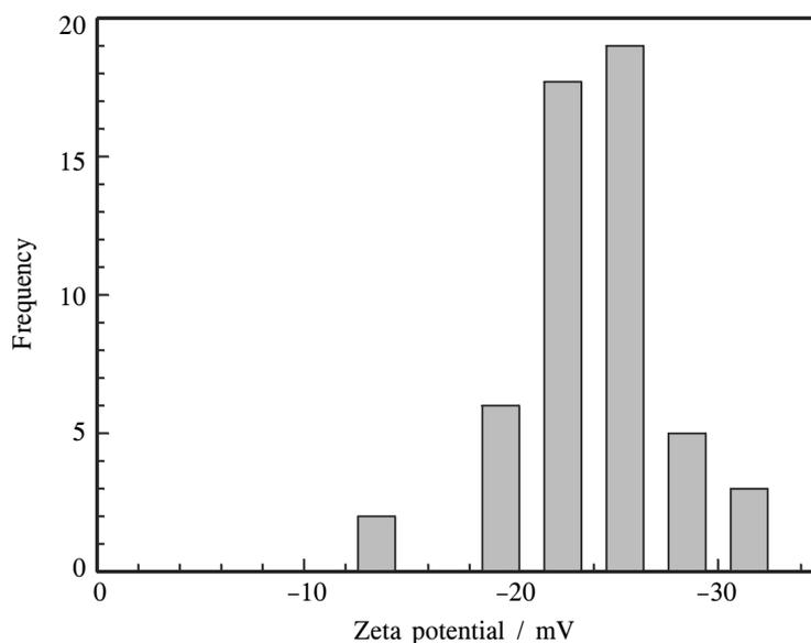
Fig. 4. Electrophoresis measurement of gelatin nanoparticle in supernatant medium at pH =5 at 25 °C. Plot of zeta potential vs. frequency is shown.
