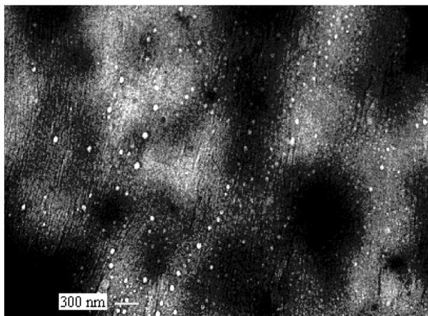
Fig. 3. TEM picture of a supernatant sample at concentration  $44 \pm 2\%$  (v/v),  $\text{pH} = 5$  at  $T = 25$  °C after staining. Particles of sizes 48nm, 65 nm and 90 nm are clearly seen in the picture.
