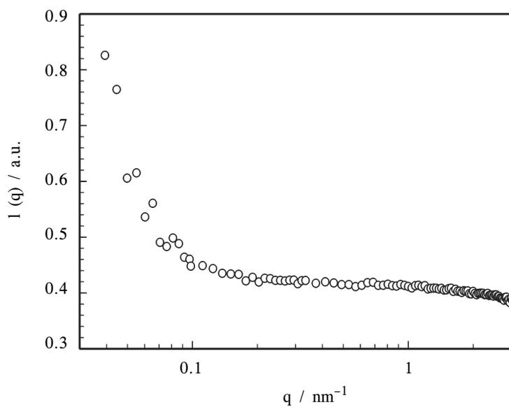
Fig. 1. SANS data for supernatant performed at 25 °C. Plot of scattering intensity ( $I$ ) versus wide range of  $\text{Log}(q)$ , ( $0.03 \text{ nm}^{-1} \leq q \leq 3.5 \text{ nm}^{-1}$ ).
