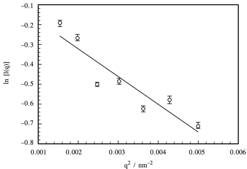
Fig. 2. SANS data for supernatant, Guinier logarithmic plot of scattering intensity versus  $q^2$  ( $q \leq 0.07 \text{ nm}^{-1}$ ).
