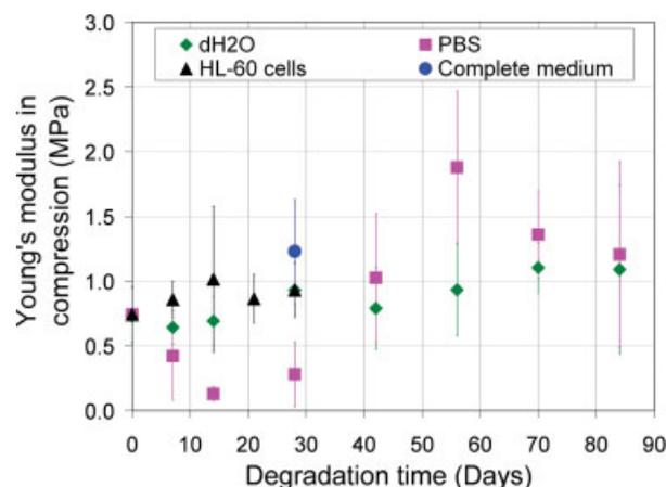
**Figure 9.** PLGA 85/15 scaffold's Young's modulus in compression tested under wet condition after degradation in different medium. [Color figure can be viewed in the online issue, which is available at [www.interscience.wiley.com](http://www.interscience.wiley.com).]
