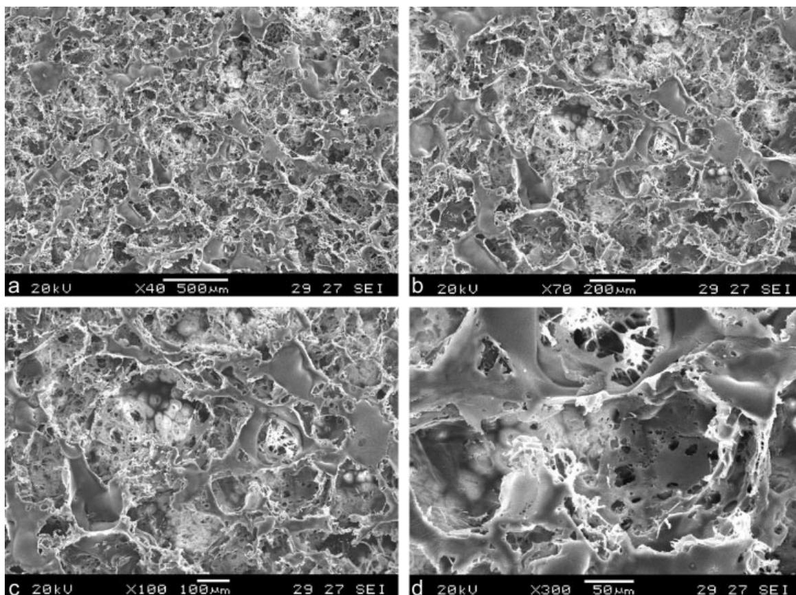
**Figure 1.** SEM images of the optimized PLGA 85/15 scaffold observed under magnification: (a)  $\times 40$ , (b)  $\times 70$ , (c)  $\times 100$ , and (d)  $\times 300$  before being used in the degradation study.
