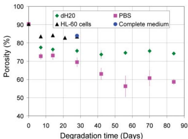
**Figure 8.** PLGA 85/15 scaffold's porosity change after degradation in different medium. [Color figure can be viewed in the online issue, which is available at [www.interscience.wiley.com](http://www.interscience.wiley.com).]
