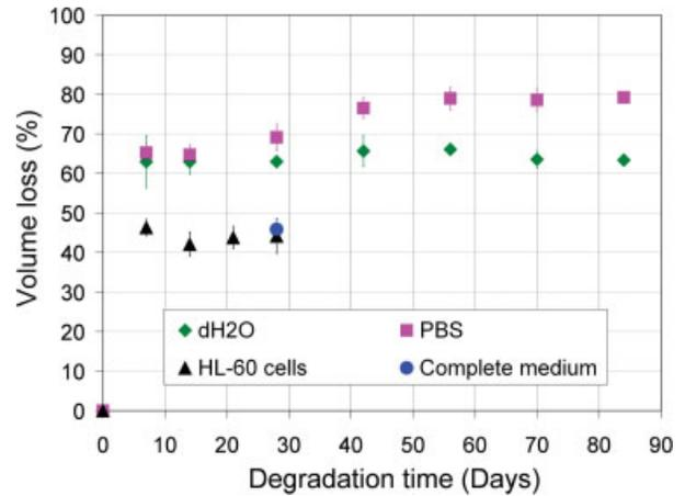
**Figure 5.** PLGA 85/15 scaffold's percentage of volume loss after degradation in different medium. [Color figure can be viewed in the online issue, which is available at [www.interscience.wiley.com](http://www.interscience.wiley.com).]
