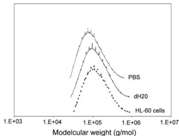
**Figure 3.** GPC curves of PLGA 85/15 scaffolds showing the effect of the different media on the MWD after a degradation time period of 28 days.
