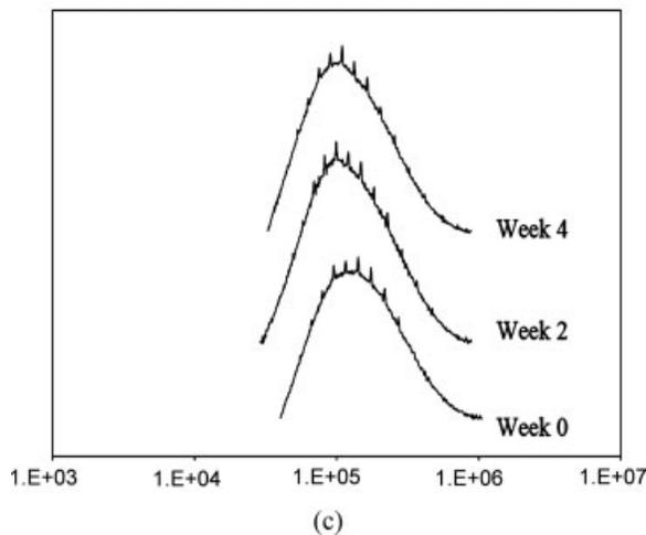
**Figure 4.** PLGA 85/15 scaffolds GPC curves showing the MWD after degradation period in: (a) dH<sub>2</sub>O, (b) PBS solution, and (c) HL-60 cells.
