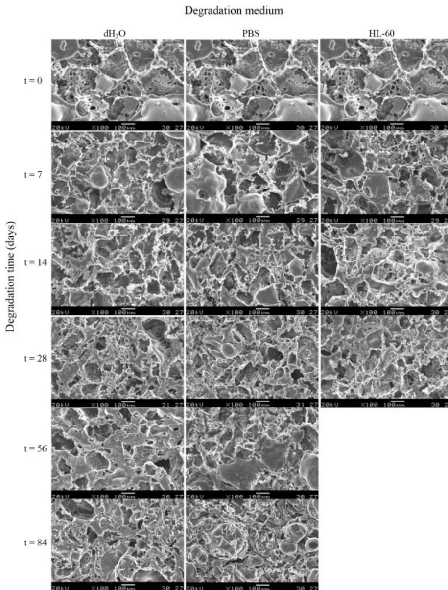
**Figure 7.** SEM images of PLGA 85/15 scaffolds observed under magnification  $\times 100$  after different degradation periods using three different media.
