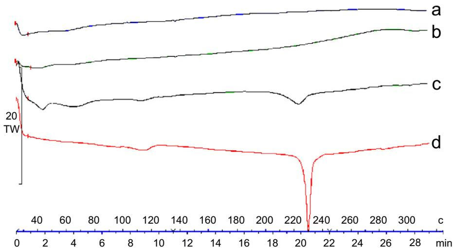
Fig. 2. DSC thermogram of PLGA (a), DM (b), physical mixture of donepezil and PLGA (c), and pure donepezil (d).
