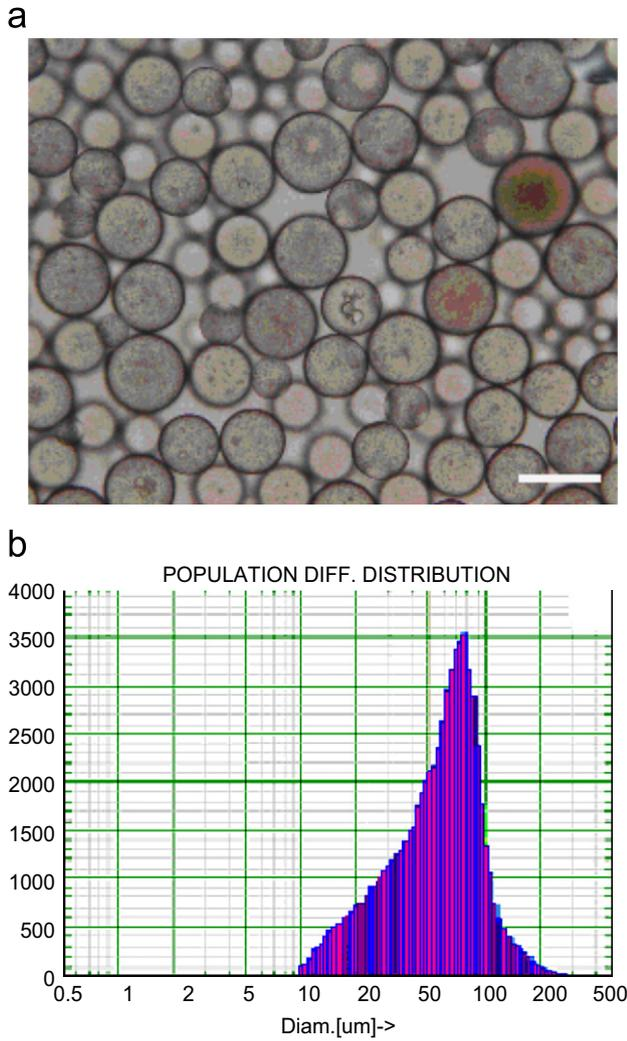
Fig. 1. The optical microscopy photograph (a, bar = 100 μm) and particle size distribution (b) of DM.
