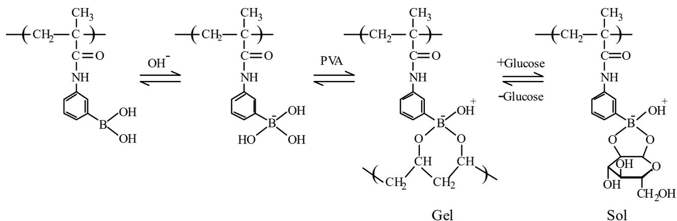
**Figure 12.3** Sol-gel phase-transition of a phenylborate polymer. At alkaline pH, phenylborate polymer interacts with poly(vinyl alcohol) (PVA) to form a gel. Glucose replaces PVA to result in transition of a gel to a sol.
