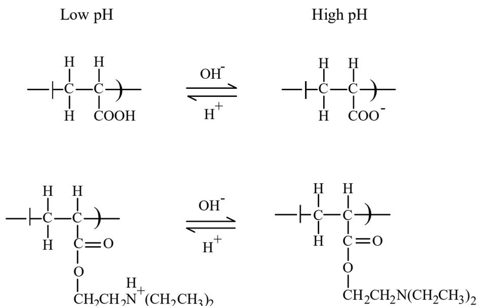
**Figure 12.5** pH-dependent ionization of polyelectrolytes. Poly(acrylic acid) becomes ionized at high pH, while poly(*N,N'*-diethylaminoethyl methacrylate) becomes ionized at low pH. Ionized polymers dissolve more in aqueous solution. Hydrogels swell more since they are not water-soluble.
