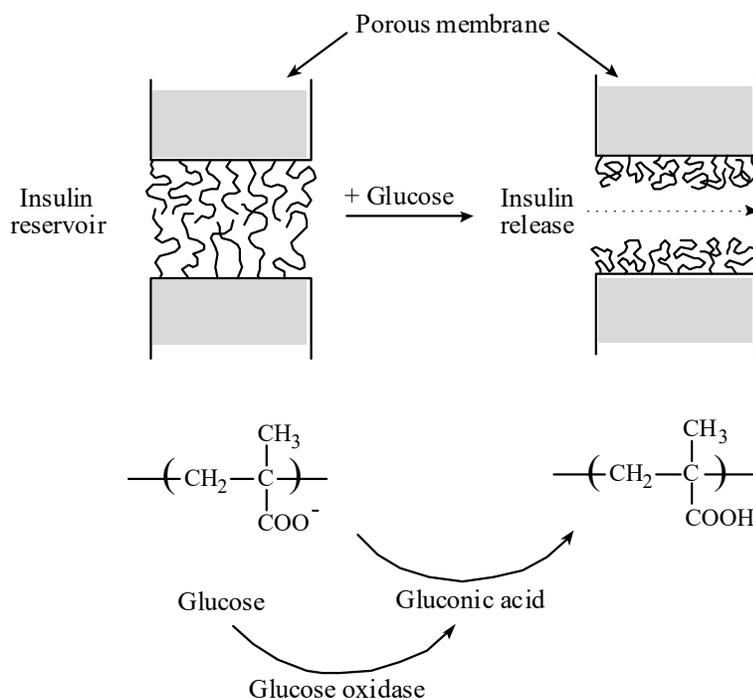
**Figure 12.7** Anionic polymer chains grafted to the surface undergo conformational changes in response to pH changes. At physiological pH, poly(methacrylic acid) (PMAA) chains are expanded due to electrostatic repulsion of carboxylate ions. As the pH decreases as a result of gluconic acid formation, the carboxylate groups are protonated and the electrostatic repulsion is reduced. This in turn causes shrinkage of the polymer chains to open pores for insulin release.
