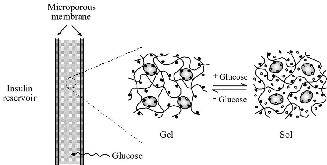
**Figure 12.2** Sol-gel phase-transition of a glucose-sensitive hydrogel. Large circles represent Con A, a glucose-binding protein. Small closed and open hexagons represent a polymer-attached glucose and a free glucose, respectively.
