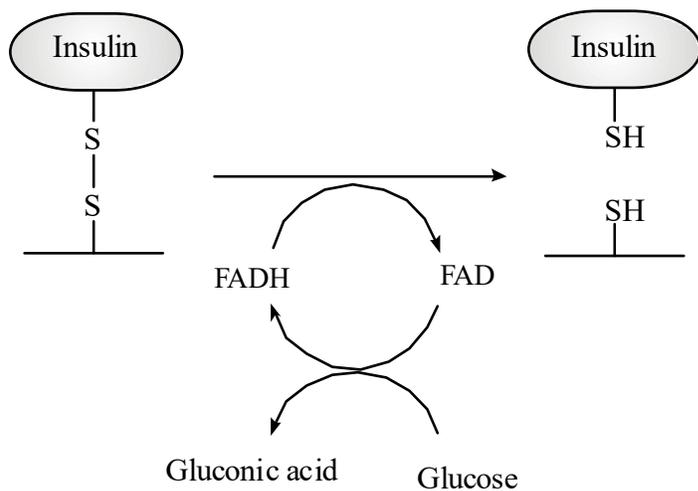
**Figure 12.10** Release of immobilized insulin in response to addition of glucose. The disulfide bond is cleaved by electrons resulting from glucose transformation to gluconic acid by glucose oxidase. This approach requires a coenzyme flavin adenine dinucleotide (FAD).
