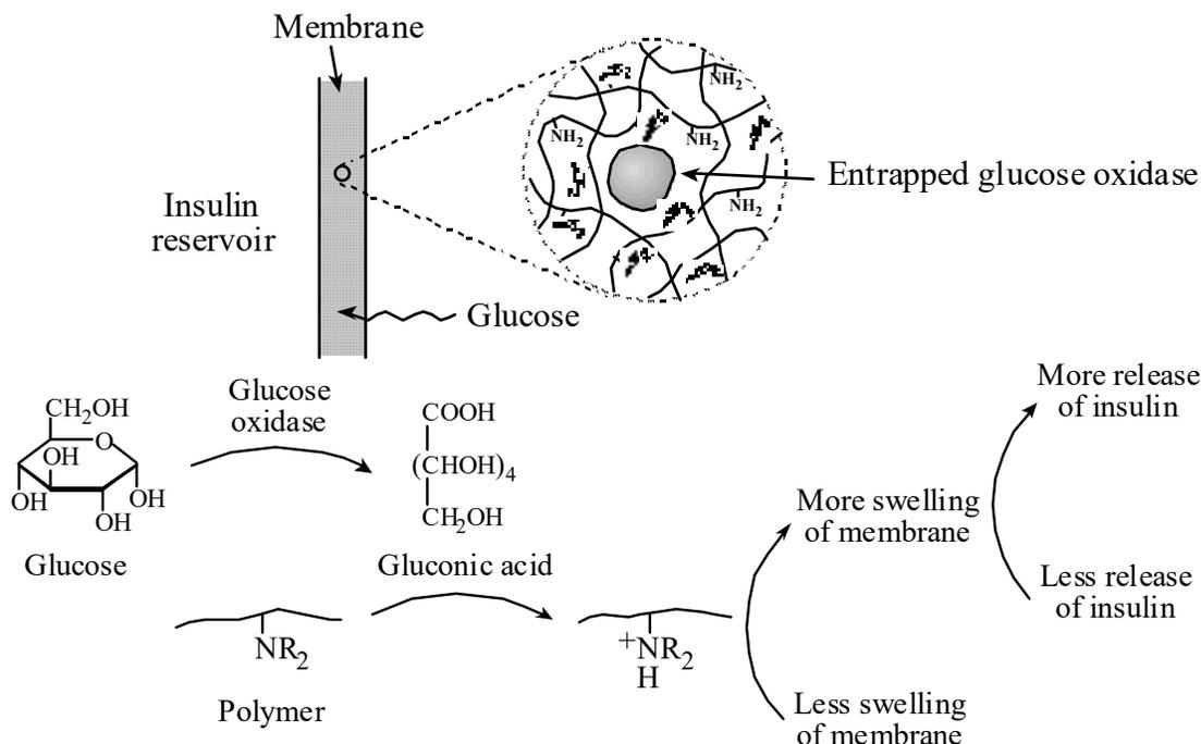
**Figure 12.6** Self-regulated insulin release membrane made of poly(*N,N'*-diethylaminoethyl methacrylate) hydrogel membrane. As glucose enters the membrane, glucose oxidase entrapped inside the membrane transforms glucose into gluconic acid, which in turn reduced the pH of the hydrogel membrane. This makes swelling of the membrane followed by more release of insulin through the membrane.
