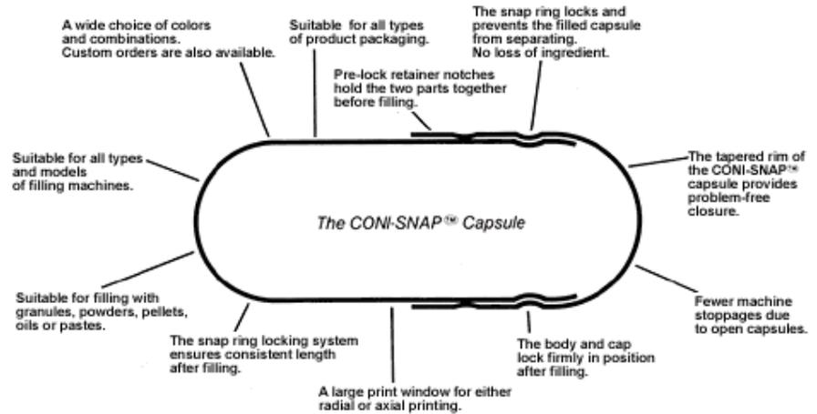
**Figure 3.1** Chart indicating the characteristics of the Coni-Snap<sup>®</sup> capsule (Cap-sugel: Pfizer, Inc.).
