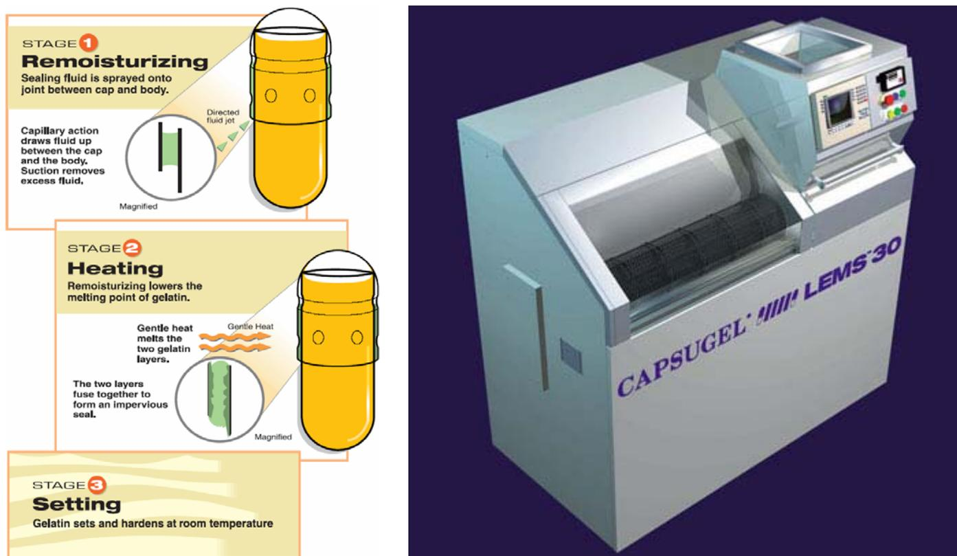
**Figure 3.5** (Left) Sealing mechanism for Licaps<sup>®</sup> capsules and (right) the Capsugel LEMS<sup>™</sup> 30 (Liquid Encapsulated Microspray Sealing) capsule-sealing equipment (Capsugel: Morris Plains, NJ).
