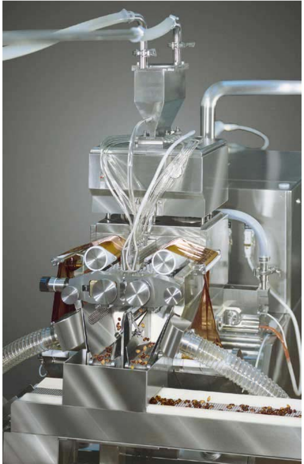
Figure 3.9 A rotary-die soft gelatin capsule filler (Pharmagel Engineering SPA: Milan, Italy)
