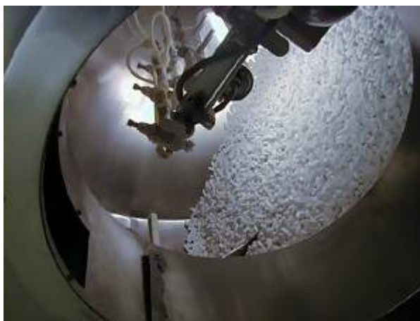
Figure 7.8 A 42-in perforated coating pan with spray nozzles (upper left) and tumbling cores (lower right).
