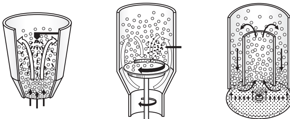
Figure 7.6 Schematic diagrams of spraying methods for coating in fluid-bed processing: top spray (left), tangential spray (center), and bottom spray (right).
