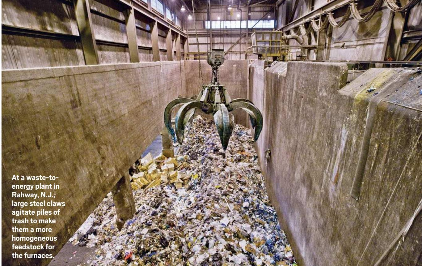
At a waste-to-energy plant in Rahway, N.J., large steel claws agitate piles of trash to make them a more homogeneous feedstock for the furnaces.
