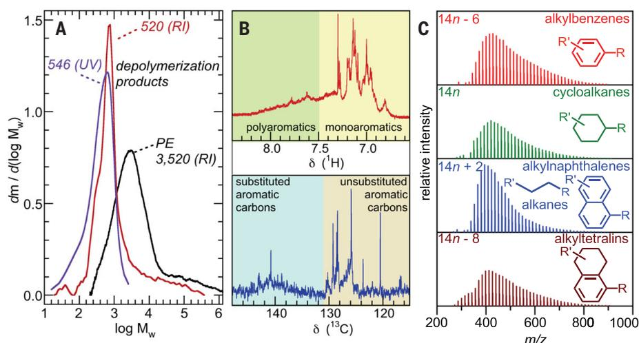
**Fig. 3. Analysis of the liquid hydrocarbon fraction from the solvent-free catalytic conversion of polyethylene.** Sample had  $M_w = 3.52 \times 10^3 \text{ g mol}^{-1}$  and was heated for 24 hours at  $280^\circ\text{C}$  (Fig. 2B, experiment 3). (A) GPC analysis, conducted using both RI and UV detectors. (B)  $^1\text{H}$  and  $^{13}\text{C}$  NMR spectra, recorded in deuterated TCE. (C) FD-MS analysis.
