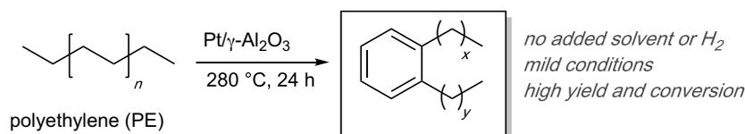
**Fig. 1. Routes to alkylbenzenes.** (A to C) Current and proposed routes to BTX (A) and the current downstream transformation of BTX to linear alkylbenzenes (B) are compared to the one-pot tandem process from polyethylene (C) reported here.
