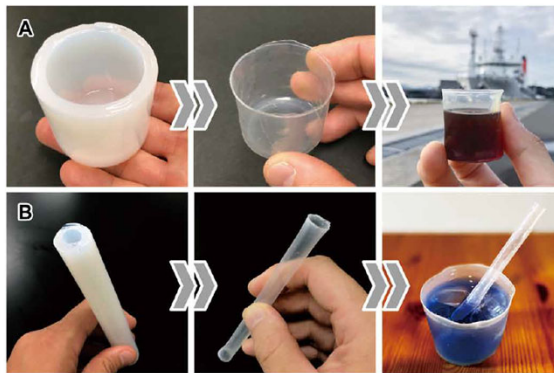
Fig. 3. Shapable nature of tPB. (A) Preparation scheme and appearance of cup-shaped tPBtex. The liquid-filled shaped tPBtex was photographed within 30 min from filling of hot coffee. (B) Preparation protocol and appearance of straw-shaped tPBtex. The liquid-filled shaped tPBtex was photographed within 30 min from filling of iced butterfly pea tea.
