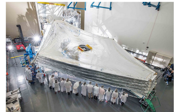
Test unit of the James Webb Space Telescope sunshield, made of aluminized Kapton
