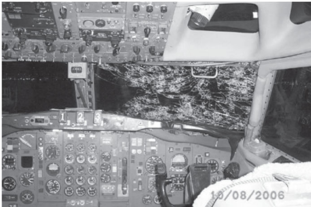
13.10 Hail damage to a cockpit window.
