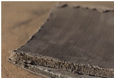
and its interior is filled with dry concrete
