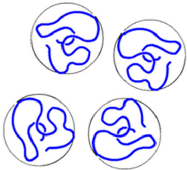
Step 2. solvated polymer molecules dispersed into a solution
