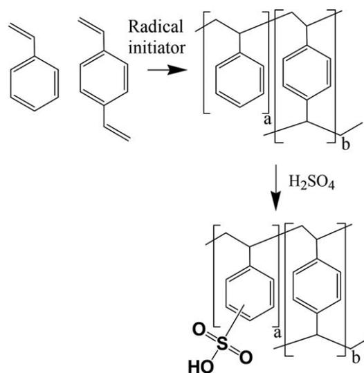
**FIGURE 3** Synthesis of Crosslinked Polystyrene Sulfonate.
