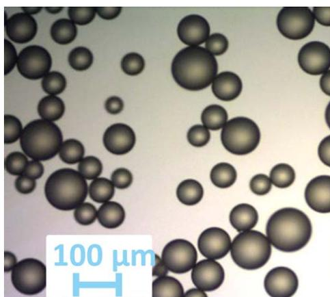
**FIGURE 9** Patiromer beads by optical microscopy. [Color figure can be viewed at [wileyonlinelibrary.com](http://wileyonlinelibrary.com)]
