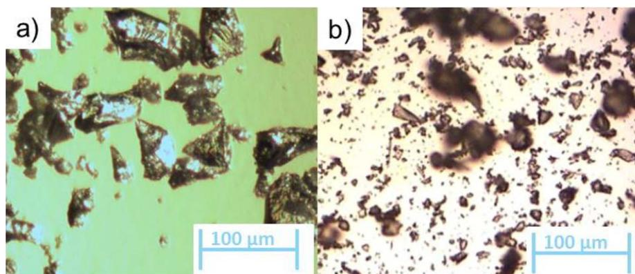
**FIGURE 4** Ground polymer morphology of a) Sevelamer; b) Kayexalate by optical microscopy. [Color figure can be viewed at [wileyonlinelibrary.com](http://wileyonlinelibrary.com)]
