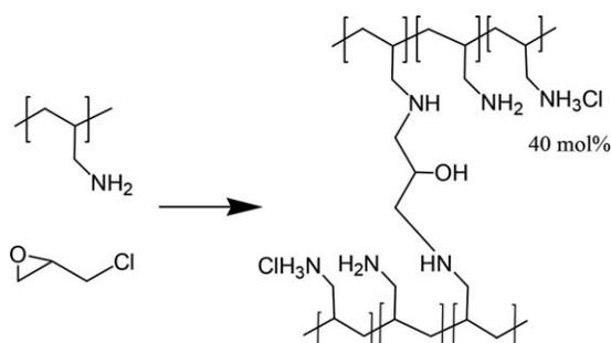
**FIGURE 5** Synthesis of Sevelamer Hydrochloride. Approximately 40% of the amine moieties are in the HCl form. Cross-linking degree is 10%.<sup>25</sup>
